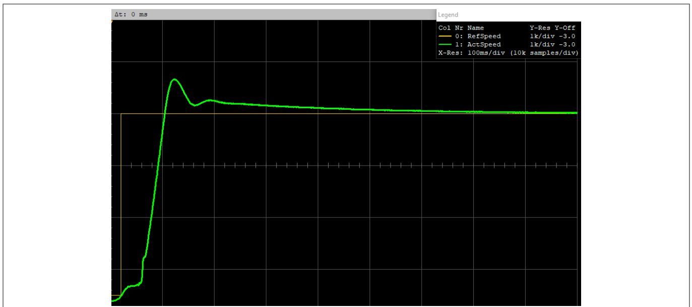
Figure 34 PI controller in time domain
