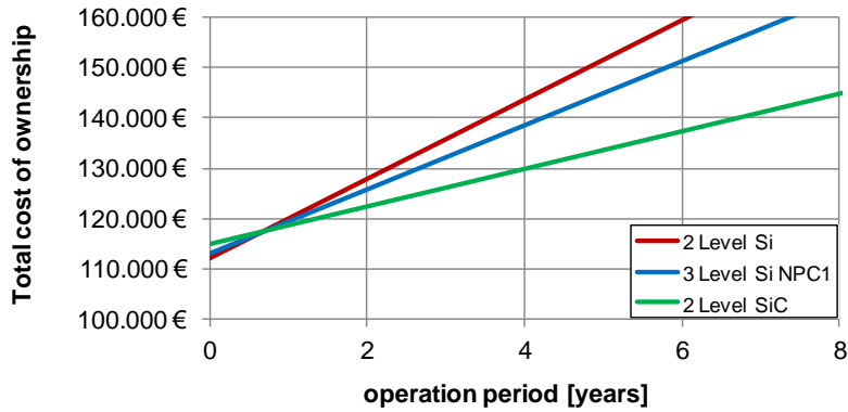
Figure 6: Total Cost of Ownership for different technical solutions, using electricity costs of 0.10 €/kWh. A 3-Level solution provides significant savings, while a SiC-based solution shows the best overall performance.
