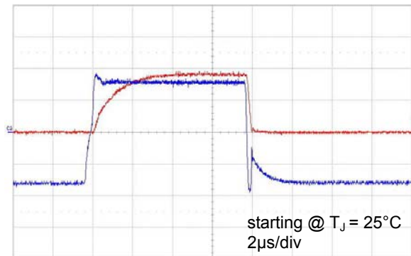
Fig. 6. Short circuit of the TCS-IGBT: gate emitter voltage (blue, 10V/div) and load current (red, 500A/div)
