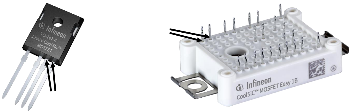
Figure 6 Example of gate-voltage measurement points
