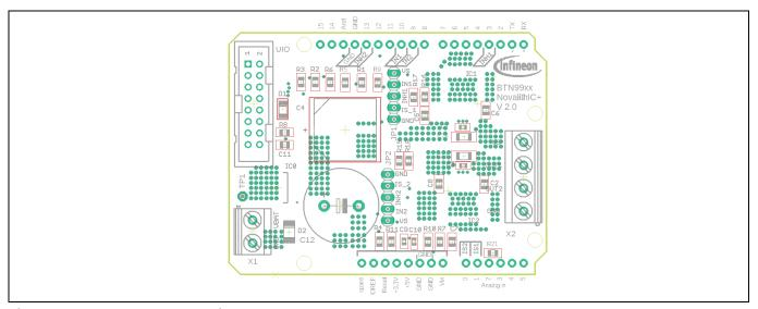
Figure 15 Components top side rev. 2.0
