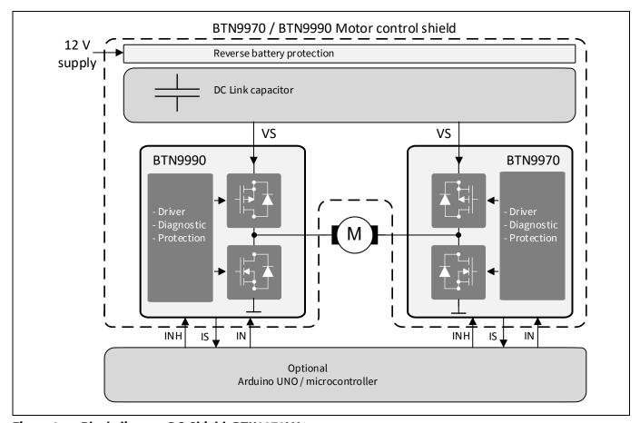
Figure 2 Block diagram DC-Shield\_BTN9970LV
