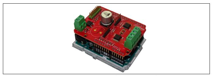
Figure 1 BTN9960/BTN9970/BTN9990 motor control shield stacked on Arduino UNO board
