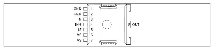
Figure 5 Pin assignment BTN99xxLV top view
