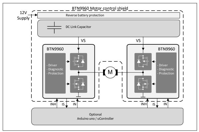
Figure 3 Block diagram DC-Shield\_BTN9960LV
