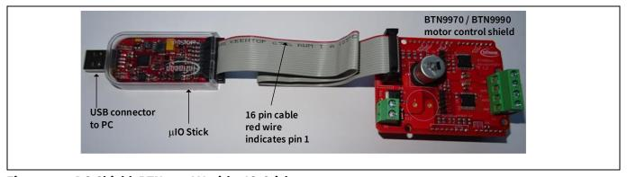
Figure 7 DC-Shield\_BTN9970LV with μIO-Stick
