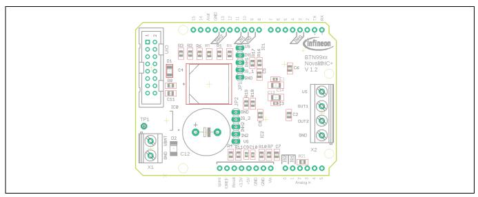
Figure 10 Components top side rev. 1.2
