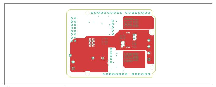
Figure 13 Inner2 layer, top view rev. 1.2
