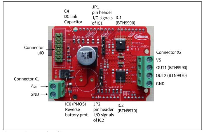
Figure 4 **Board top view with connectors**
