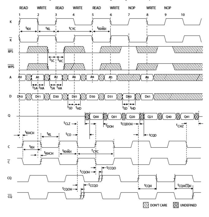
Figure 4. QDR-II/II+ Burst of Two Timing Showing Read Latency of Two
