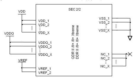
Figure 40. QDR II/II+/II+Xtreme-DDR II/II+/II+Xtreme (Supply Pins) Reference Schematic
