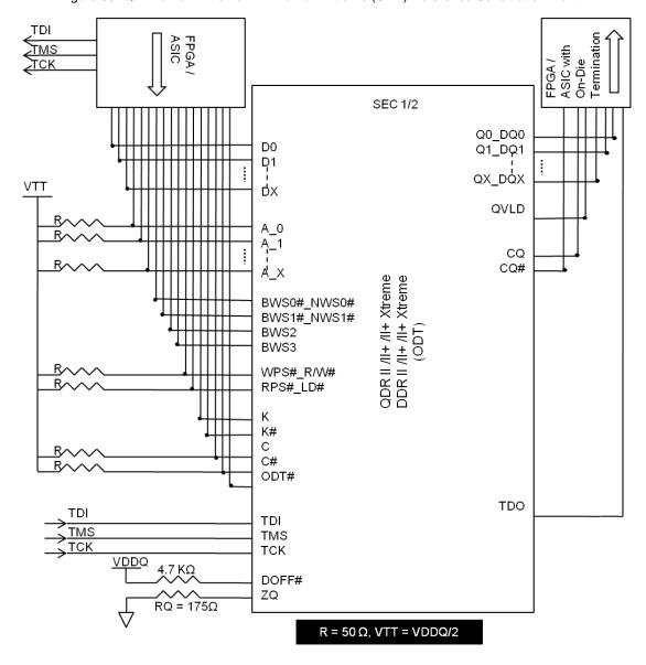
Figure 39. QDR II/II+/II+Xtreme-DDR II/II+/II+Xtreme (ODT) Reference Schematic—Part 2
