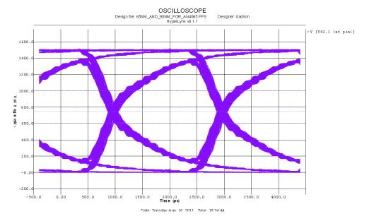
Figure 27. Eye Diagram for Series Resistors Termination Case
