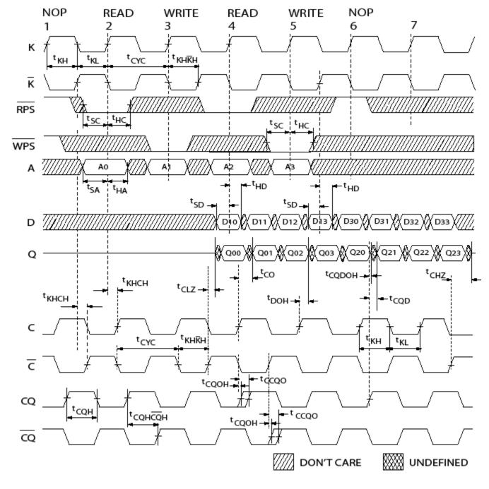
Figure 5. QDR-II/II+ Burst of Four Timing Showing Latency of Two
