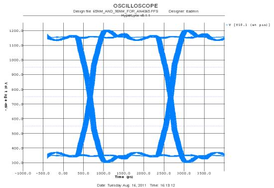
Figure 20. Eye Diagram for R1 = 50  $\Omega$  Active Pull-Up Termination Case
