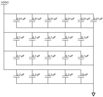
Figure 43. Decoupling Capacitor Recommendation for  $V_{TT}$
