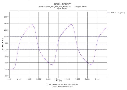
Figure 26. Using  $50-\Omega$  Series Resistances on Both Ends
