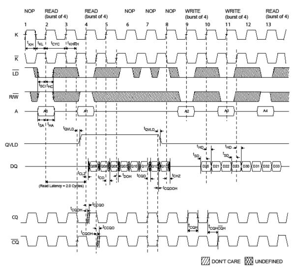
Figure 7. DDR II/II+ Burst of Four Timing Showing Latency of Two
