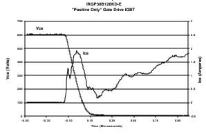
Figure 8. Vce & Ice vs. time dv/dt turn-on current
