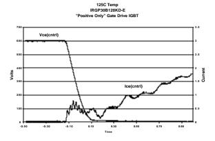
Figure 11. Vce & Ice vs. time dv/dt turn-on current test -diode only
