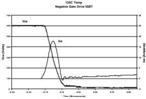
Figure 7. Vce & Ice vs. time dv/dt turn-on current
