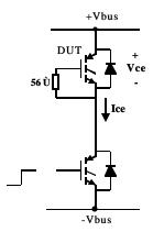
Figure 6. dv/dt turn-on current test circuit
