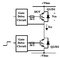
Figure 2. Half Bridge Circuit
