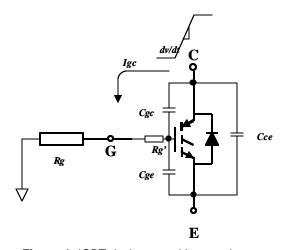
Figure 1. IGBT device parasitic capacitances
