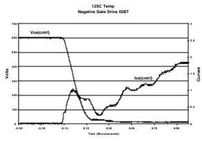
Figure 10. Vce & Ice vs. time dv/dt turn-on current test -diode only
