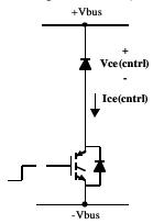
Figure 9. dv/dt turn-on current test circuit - diode only
