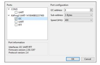
To establish the I2C communication between the Tuner and target device, configure the Tuner communication parameters to match the parameters of the device EzI2C settings.
