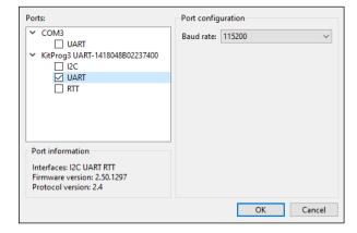
To establish the UART communication between the Tuner and target device, configure the Tuner communication parameters to match the parameters of the device UART settings.
