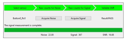
The progress bar provides graphical guidance to the user to complete the SNR measurement. The bar displays the progress and user-addressed relevant messages.
