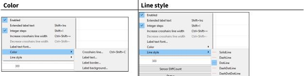
Vertical marker lines – When you left-click, the Tuner adds a Vertical marker line with a value equal to the X coordinate of the mouse cursor synchronously on all four charts – Sensor Data, Sensor Signal, Status, and Position regardless of their scale and shift. Press the [Esc] key to erase all previously drawn Vertical marker lines. You can change the characteristics of Vertical marker lines or disable them in the submenu Chart settings > Vertical marker lines.
