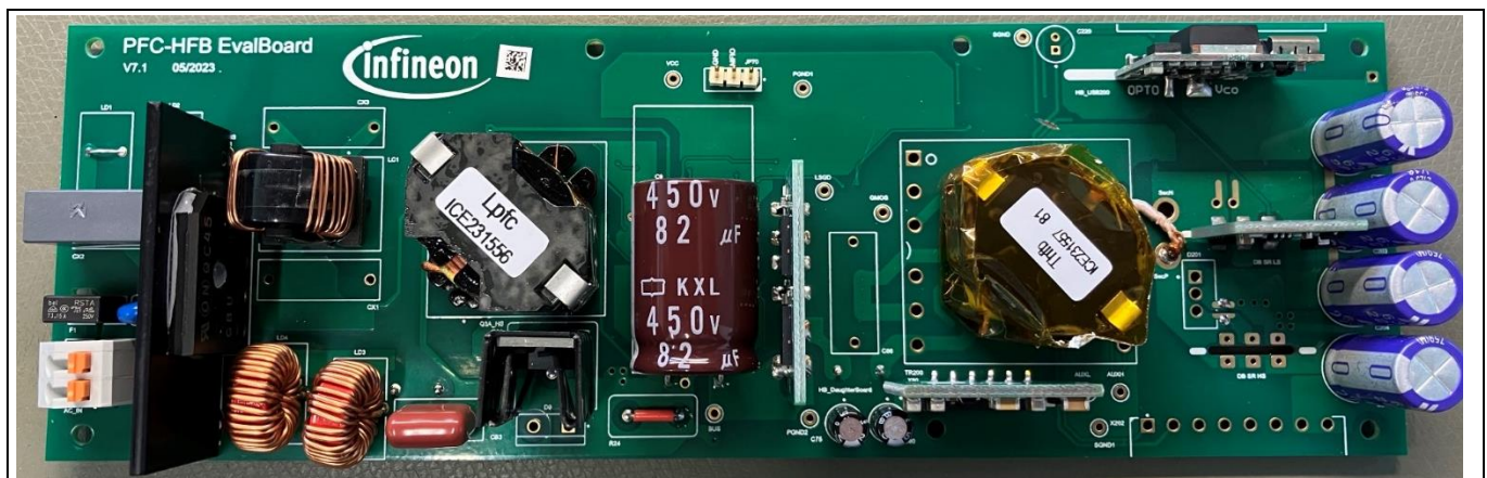
Figure 2 Evaluation board with daughter boards
