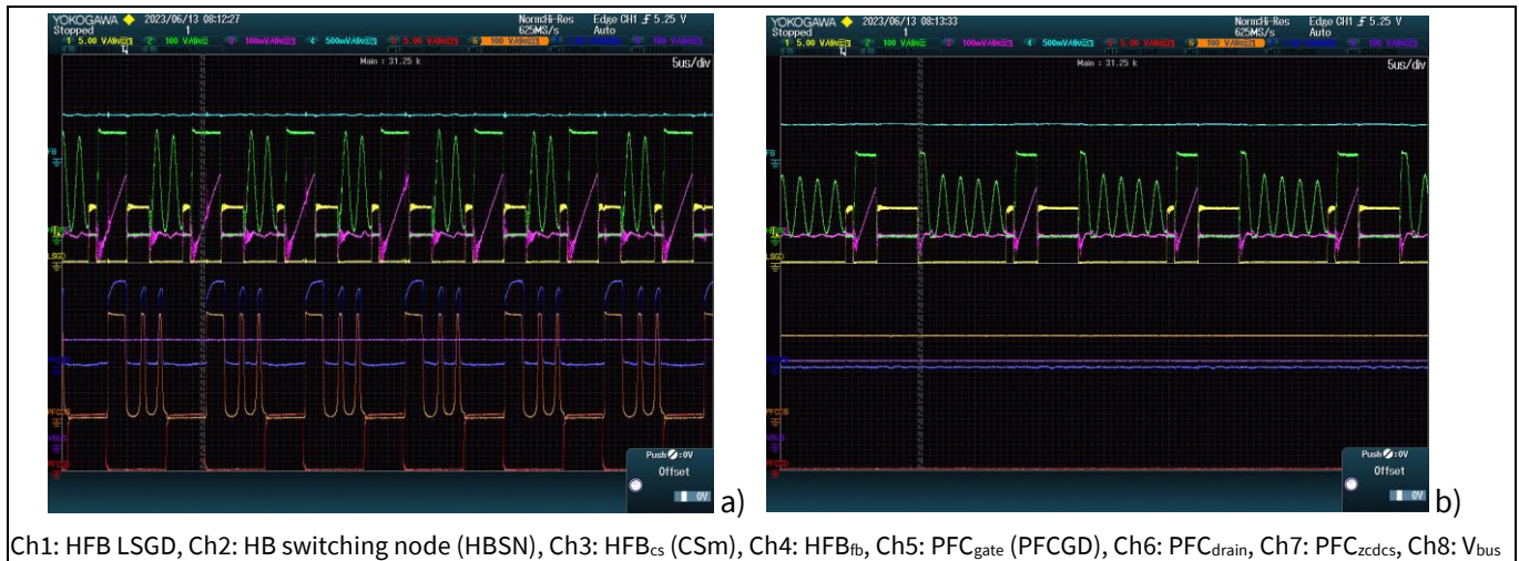
Figure 17 Continuous operation mode with HFB in ZV-RVS mode: a) PFC switching at third valley at 115 V input and 48 V 2 A output, and b) PFC disabled at 230 V, 28 V 1 A output
