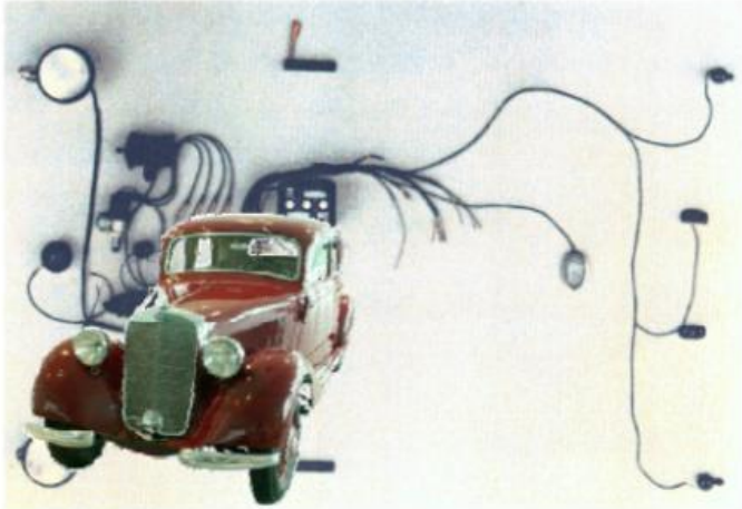
Harness 1949 ca. 40 wires ca. 60 connectors
