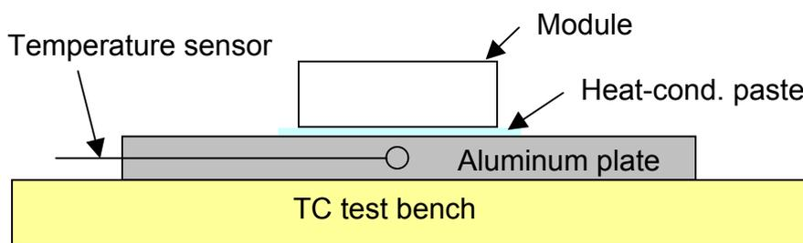
Fig 1: Test set-up
