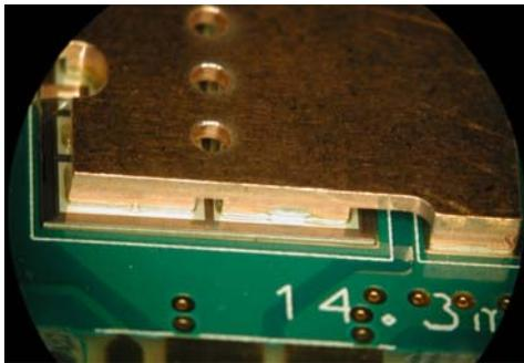
Fig. 6 A side view of Cu-clip IGBT
