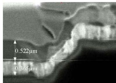
Fig. 2 SFM coverage over the passivation layer.
