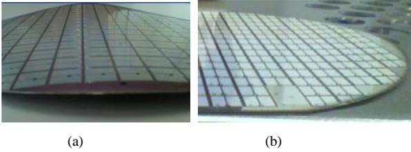
Fig. 3 Standard process could lead to (a) compressive or (b) tensile stressed wafers.
