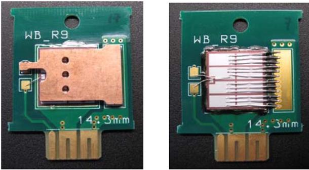
(a) Cu-clip IGBT. (b). Wire-bonded IGBT
