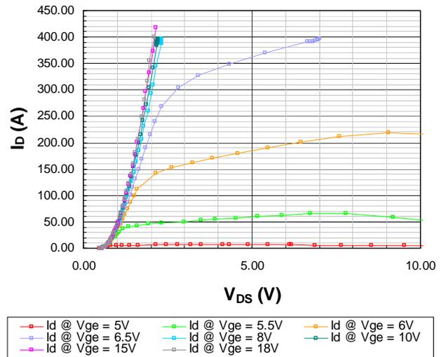
Fig. 8 Output Characteristics at 25C at various Vge.
