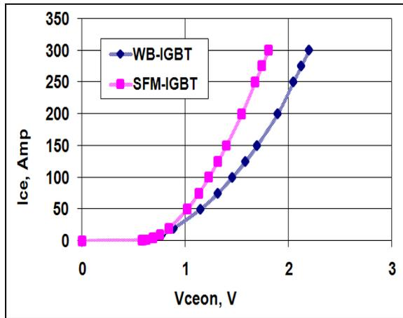
Fig. 9 I-V curves for WB-IGBT and SFM-IGBT.
