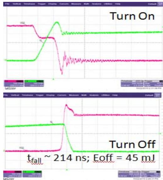
Fig. 12 Turn-on and turn-off waveforms of SFM - IGBT with Cu-clip. ( $V_{cc}=400V$ ,  $I_c=300A$ , 25°C)
