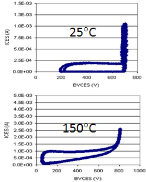
Fig. 11 Breakdown voltages at 150C for SFM- IGBTs with Cu clip.
