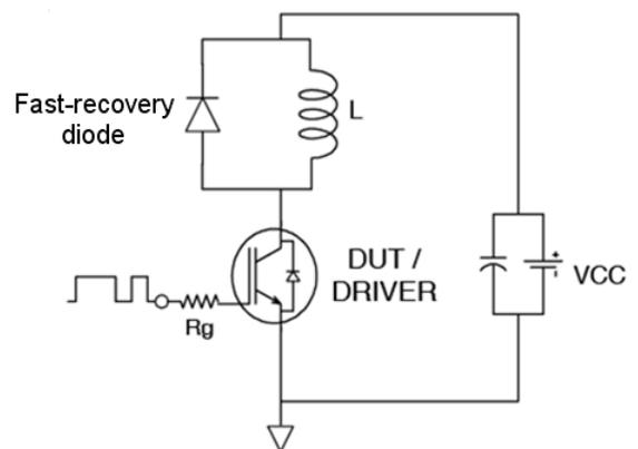
Fig. 5 Test circuit used for the measurements of the switching characteristics of IGBT and MOSFET.
