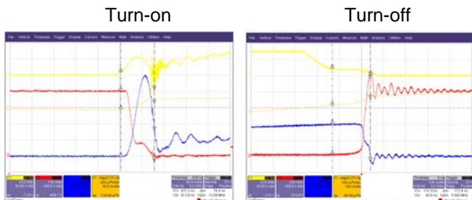
Fig. 7 Switching waveforms of a SJ MOSFET at Ic=10A, Vcc=400V and 150°C
