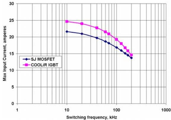
Fig. 8 Comparison of maximum input current at various switching frequencies for COOLiRIGBT™ and SJ MOSFET at 150°C for ZVS applications.
