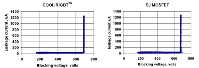
Fig. 4 Comparison of the reverse blocking characteristics of COOLiRIGBT™ and SJ MOSFET.
