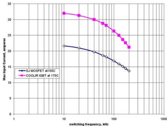
Fig. 9 Maximum input current at 200 kHz is increased by 50% for COOLiRIGBT™ with  $T_{jmax}=175^{\circ}\text{C}$  comparing with 14A for SJ MOSFET with  $T_{jmax}=150^{\circ}\text{C}$ .
