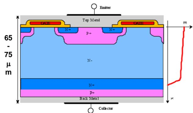
Fig. 1 Punch-Through thin IGBT structure
