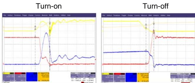
Fig. 6 Switching waveforms of COOLiRIGBT™ at Ic=10A, Vcc=400V and 150°C
