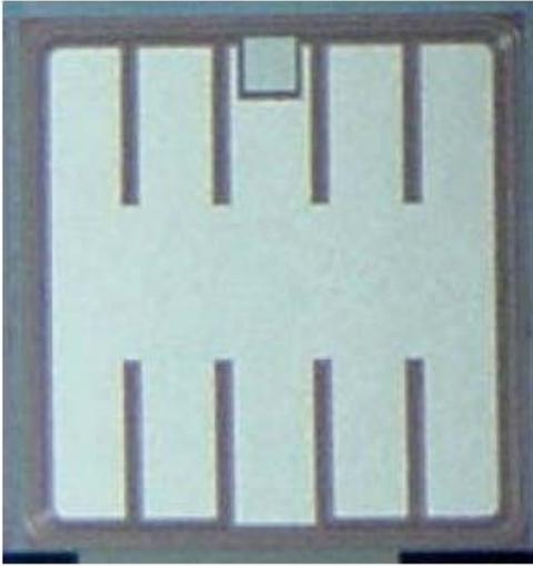
Fig. 2 Photograph of a high speed thin IGBT
