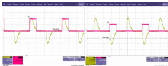
Fig 15: Vg1, Vg2: Gate signal Q1 and Q2 and line current under RC load R=22 ohm C=470uF.
