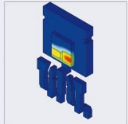
P-TO252-3-1 without mold compound with P_V = 3 W for determining the R_{thj-c}
