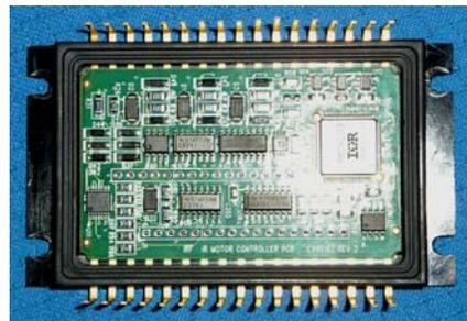
**Figure 12 Control and Gate Drive Circuitry**
