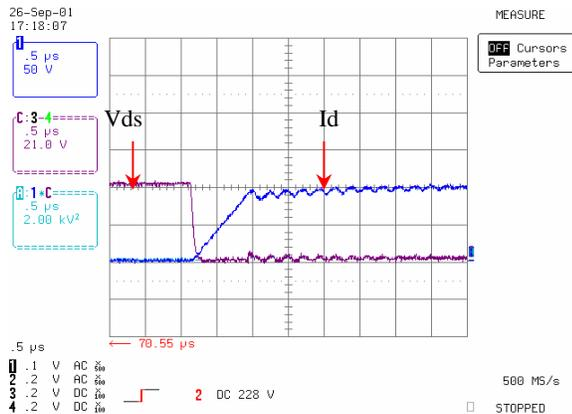
Figure 20: Measured Vds and Id during Turn-on
