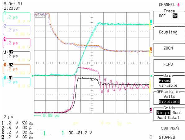
Figure 10: Channel 1 2 4 IRFP2907 with 80nH external inductance  $V_{bus}=42.7V$
