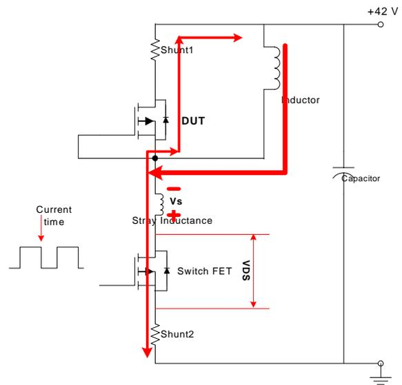
Figure 8: Transient Process During Turn-off
