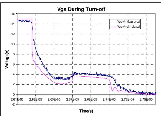
Figure 3: Comparison of Vgs during turn-off
