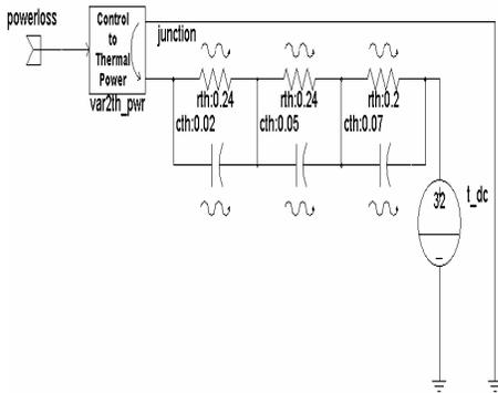
Figure 14: Schematic of the Thermal Model
