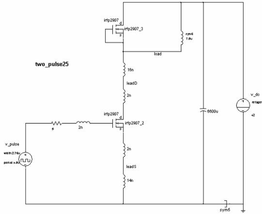
Figure 1: Schematic of the two-pulse test circuit
