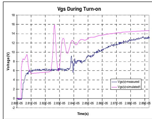
Figure 5: Comparison of Vgs during turn-on
