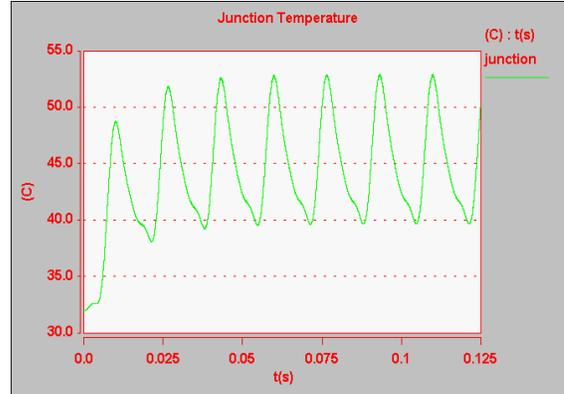
Figure 15: Tjunction Response of one MOSFET
