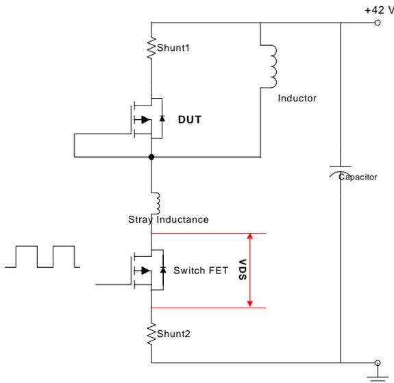
Figure 6: Circuit Diagram of the Two Pulse Test
