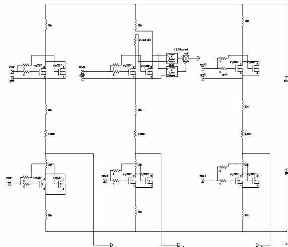
Figure 12: Schematic of the Inverter
