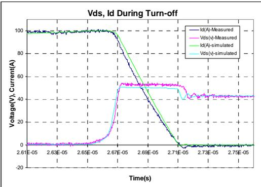
Figure 2: Comparison of Vds and Id during turn\_off
