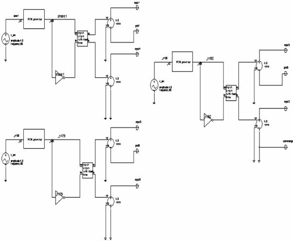
Figure 13: Schematic of the three-phase PWM Signal Generator
