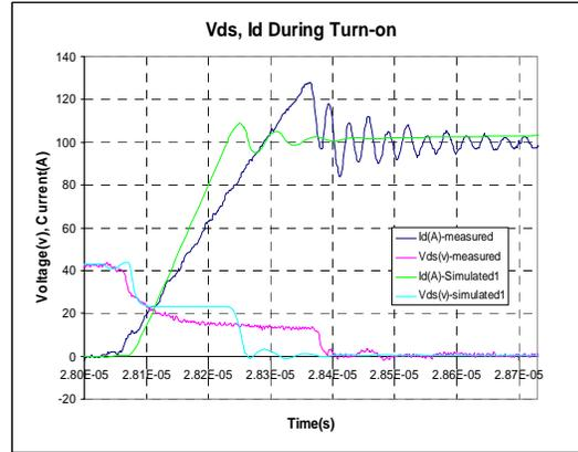
Figure 4: Comparison of Vds and Id during turn-on
