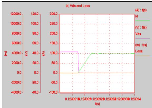
Figure 19: Vds and Id during Turn-on ( $0.5 \mu\text{s} / \text{div}$ )
