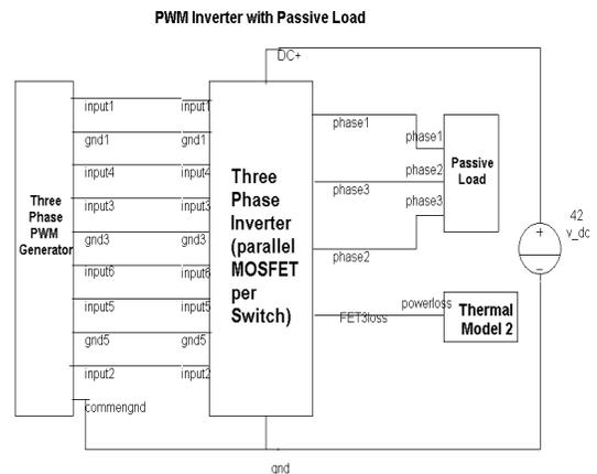
Figure 11: System Schematic
