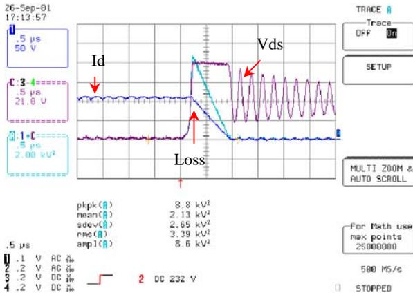
Figure 18: Measured Vds and Id During Turn-off
