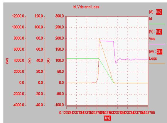
Figure 17: Vds and Id During turn-off ( $0.5 \mu S /div$ )
