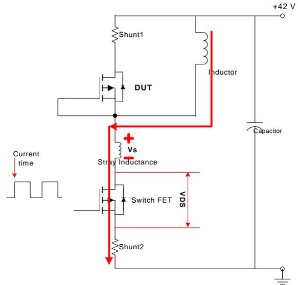
Figure 7: Transient Process During Turn-on
