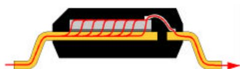
Fig. 1a A Typical Mosfet Device (SO8) showing the thermal and electrical path.
