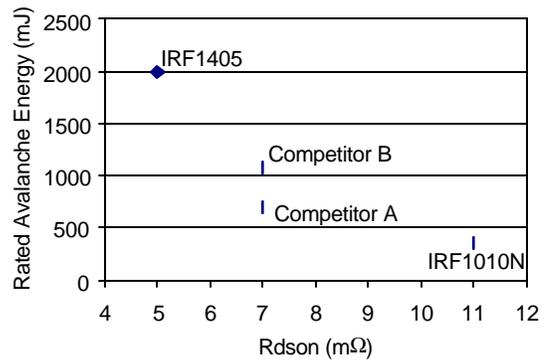
Figure 3. Rated avalanche energy versus  $R_{DS(on)}$ , illustrating high ruggedness and low  $R_{DS(on)}$  for equivalent die sizes.
