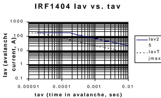
Figure 5. Curve of  $I_{av}$  vs.  $t_{av}$  for IRF1404
