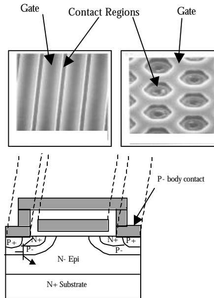
Figure 1. Photo of stripe versus cell topologies and cross-section of power MOSFET showing parasitic bipolar transistor.
