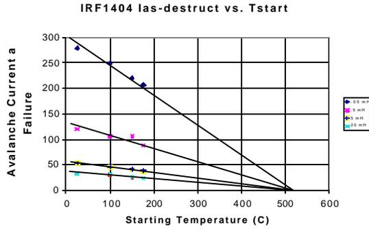
Figure 4.  $I_{as}$ -destruct versus  $T_{start}$  for IRF1404.
