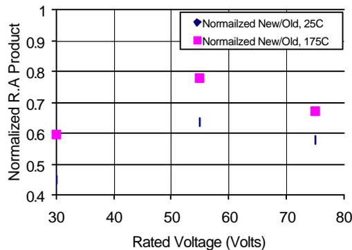
Figure 2. Normalized R.A product versus rated breakdown voltage. Measurements have been made at  $V_{gs} = 10V$  and package resistance has been subtracted.
