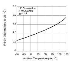
Figure 4. Typical Normalized On-Resistance
