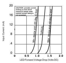
Figure 6. Input Characteristics (Current Controlled)
