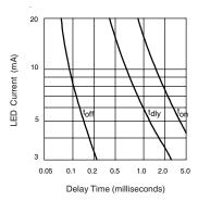
Figure 7. Typical Delay Times
