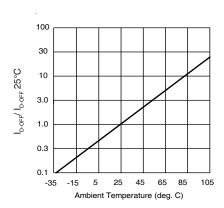
Figure 5. Typical Normalized Off-State Leakage
