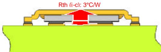
Fig. 1b A DirectFET™ Mosfet device showing the main thermal resistances
