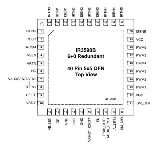
Figure 1: IR3590B Package Top View
