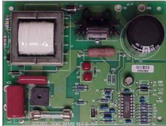
Figure 5 - Multiplier Based 250W Demo Board
