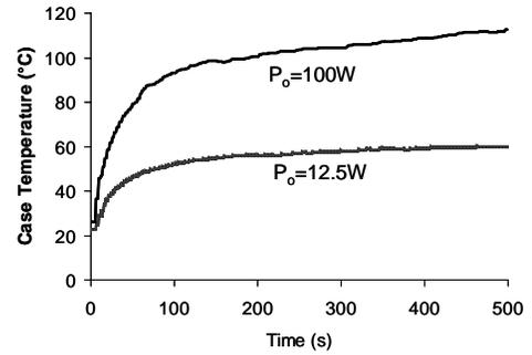
Fig. 11. The temperature measurement of the device without heatsink..
