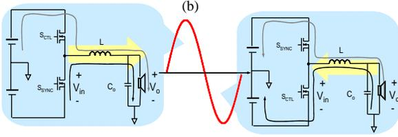
Fig. 8. The variations of power flow and operation points of a class-D audio amplifier.
