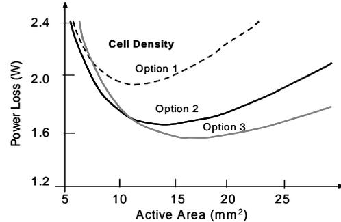
Fig. 6. Optimizing devices for isolated DC-DC converter.
