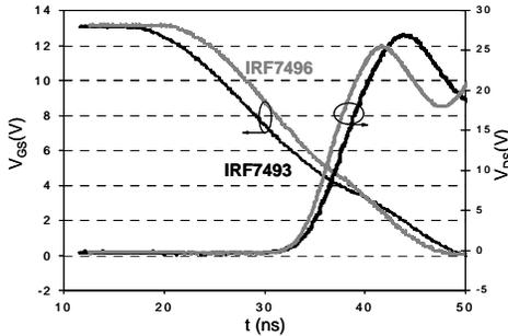
Fig. 5. The measured waveforms of the  $V_{GS}$  and  $V_{DS}$  for the verification of loss modeling.
