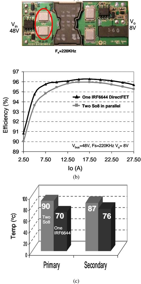
Fig. 10. Measure efficiency and device temperature for HB unregulated converter: (a) the picture of the DC bus converter, (b) measured efficiency and (c) measured device temperature.
