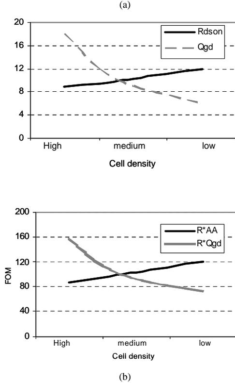
Fig. 1. Examples of MOSFET parameters as a function of cell density: (a)  $R_{ds(on)}$  and  $Q_{gd}$ ; (b)  $R_{ds(on)} \cdot Q_{gd}$  and  $R \cdot AA$ .
