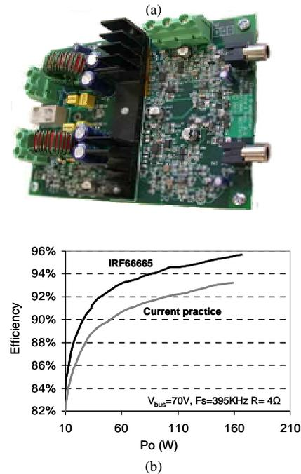
Fig. 12. Prototype and measured efficiency of class D audio amplifier: (a) the photograph of the class D audio amplifier, (b) the measured efficiency.
