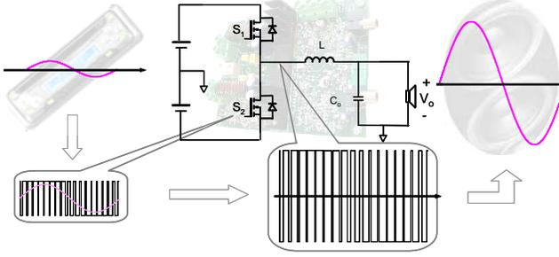
Fig. 7. Another typical application addressed in this paper--- class D audio amplifier.
