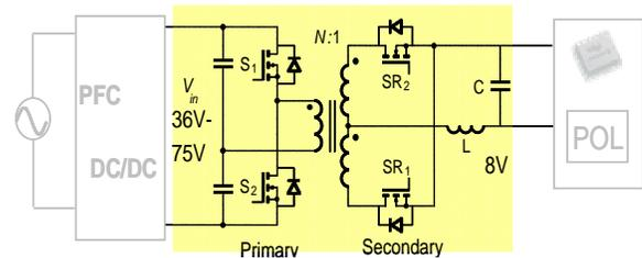
Fig. 4. The typical application addressed in this paper--- non-regulated DC bus converter.
