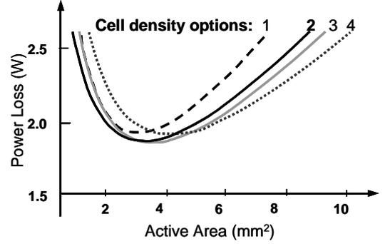
Fig. 9. Optimizing devices for class D audio amplifier.
