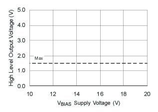
Figure 16B. High Level Output Voltage vs. Supply Voltage (I<sub>O</sub> = 0 mA)
