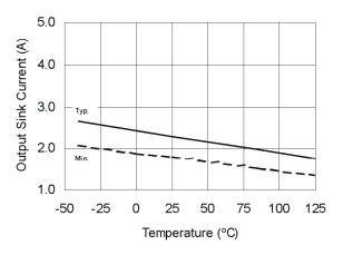
Figure 26A. Output Sink Current vs. Temperature
