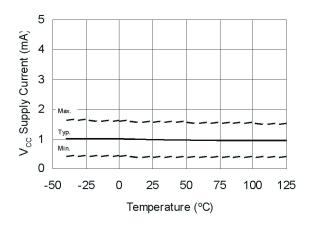
Figure 20A. V<sub>cc</sub> Supply Current vs. Temperature
