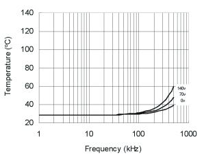
Figure 39. IRS21814s vs. Frequency (IRFBC20),  $\rm R_{\rm gate}$  =33  $\Omega,\,\rm V_{\rm CC}$  =15 V
