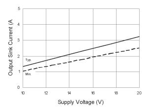
Figure 26B. Output Sink Current vs. Supply Voltage
