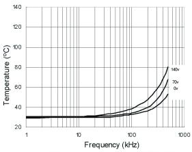
Figure 40. IRS21814s vs. Frequency (IRFBC30),  ${\rm R_{\rm nate}}\text{=}22~\Omega,~{\rm V_{\rm cc}}\text{=}15~{\rm V}$
