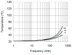
Figure 32. IRS21814 vs. Frequency (IRFBC30),  ${\rm R_{\rm oate}}\text{=}22~\Omega\,,\,{\rm V_{\rm cc}}\text{=}15~{\rm V}$
