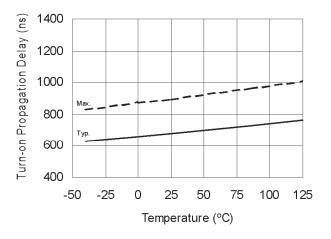
Figure 6A. Turn-On Propagation Delay vs. Temperature
