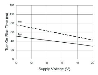
Figure 9B. Turn-On Rise Time vs. Supply Voltage
