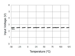
Figure 12A. Logic "1" Input Voltage vs. Temperature
