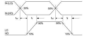
Figure 1: Input/Output Timing Diagram
