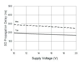
Figure 8B. SD Propagation Delay vs. Supply Voltage
