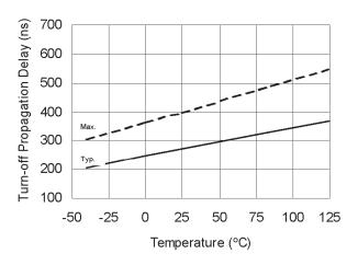
Figure 7A. Turn-Off Propagation Delay vs. Temperature
