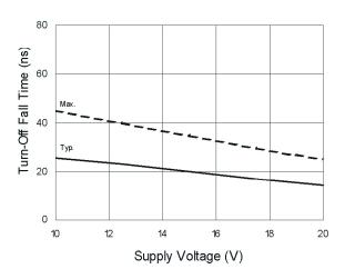
Figure 10B. Turn-Off Fall Time vs. Supply Voltage
