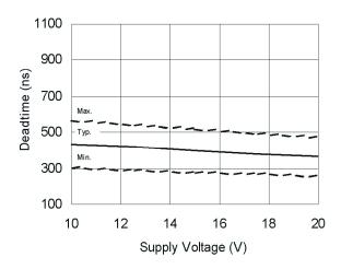
Figure 11B. Deadtime vs. Supply Voltage
