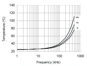
Figure 36. IRS2181s vs. Frequency (IRFBC30),  $\rm R_{\rm gate}$  =22  $\Omega$  ,  $\rm V_{\rm CC}$  =15 V
