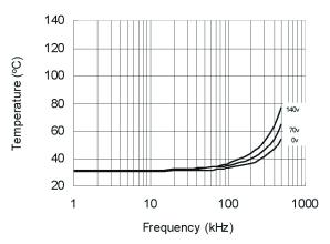
Figure 35. IRS2181s vs. Frequency (IRFBC20),  $R_{\text{oate}} \!=\! \! 33~\Omega,\, V_{\text{CC}} \! =\! \! 15~\text{V}$
