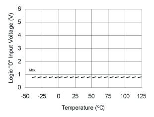
Figure 13A. Logic "0" Input Voltage vs. Temperature
