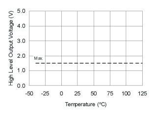
Figure 16A. High Level Output Voltage vs. Temperature ( $I_0 = 0$  mA)
