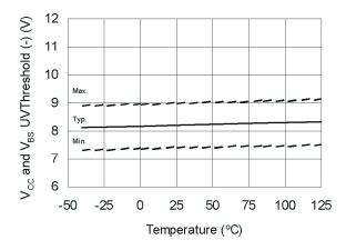
Figure 24.  $V_{\rm CC}$  and  $V_{\rm BS}$  Undervoltage Threshold (-) vs. Temperature
