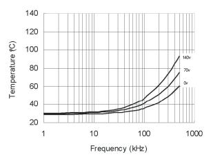
Figure 29. IRS2181 vs. Frequency (IRFBC40),  $\rm R_{gate}$  =15  $\Omega,\,\rm V_{CC}$  =15 V
