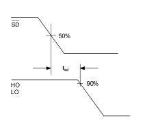
**Figure 3: Shutdown Waveform Definitions**
