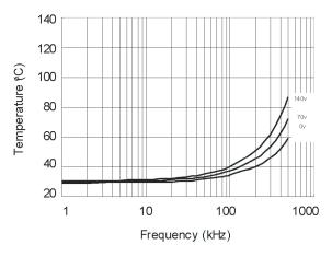
Figure 28. IRS2181 vs. Frequency (IRFBC30),  $\rm R_{\rm gate}$  =22  $\Omega,\,\rm V_{\rm CC}$  =15 V
