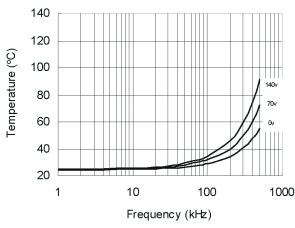
Figure 33. IRS21814 vs. Frequency (IRFBC40),  $\rm R_{\rm tate}$  =15  $\Omega$  ,  $\rm V_{\rm cc}$  =15 V
