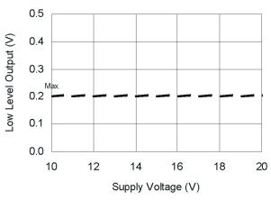
Figure 17B. Low Level Output vs. Supply Voltage
