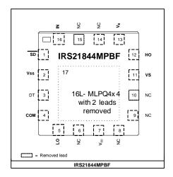
Central exposed pad (17) is internally connected to ground. It is recommended to connect the central exposed pad to COM externally for better electrical performance.
