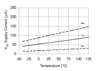
Figure 19A. V<sub>BS</sub> Supply Current vs. Temperature
