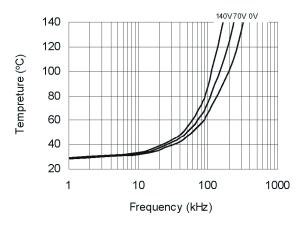
Figure 38. IRS2181s vs. Frequency (IRFPE50),  $\rm R_{gate}$  =10  $\Omega,\,\rm V_{CC}$  =15 V
