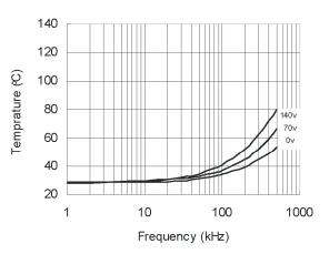
Figure 27. IRS2181 vs. Frequency (IRFBC20),  $\rm R_{\rm gate} = 33~\Omega,~V_{\rm CC} = 15~V$
