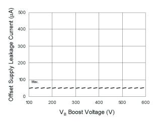
Figure 18B. Offset Supply Leakage Current vs.  $V_{\rm B}$  Boost Voltage
