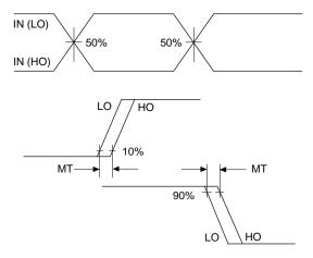
Figure 5: Delay Matching Waveform Definitions
