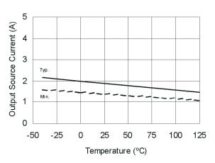
Figure 25A. Output Source Current vs. Temperature
