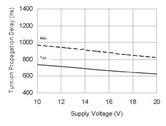
Figure 6B. Turn-On Propagation Delay vs. Supply Voltage
