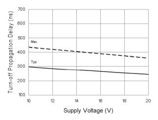
Figure 7B. Turn-Off Propagation Delay vs. Supply Voltage
