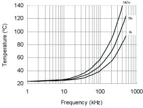
Figure 34. IRS21814 vs. Frequency (IRFPE50),  $\rm R_{gate}$  =10  $\Omega,\,\rm V_{CC}$  =15 V
