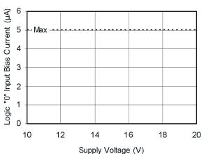
Figure 22B. Logic "0" Input Bias Curremt vs. Voltage
