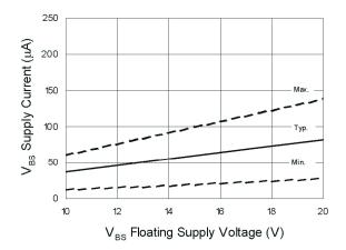
Figure 19B.  $V_{\rm BS}$  Supply Current vs.  $V_{\rm BS}$  Floating Supply Voltage
