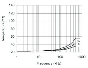
Figure 31. IRS21814 vs. Frequency (IRFBC20),  ${\rm R_{\rm qate}}\text{=}33~\Omega,\,{\rm V_{\rm CC}}\text{=}15~{\rm V}$
