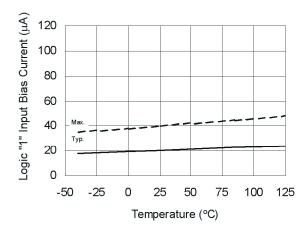
Figure 21A. Logic "1" Input Bias Current vs. Temperature
