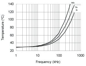
Figure 30. IRS2181 vs. Frequency (IRFPE50),  $\rm R_{\rm gate}$  =10  $\Omega,\,\rm V_{\rm CC}$  =15 V
