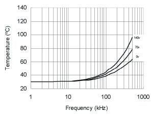
Figure 41. IRS21814s vs. Frequency (IRFBC40),  $\rm R_{\rm uate}$  =15  $\Omega,\,\rm V_{\rm CC}$  =15 V
