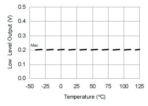
Figure 17A. Low Level Output vs. Temperature
