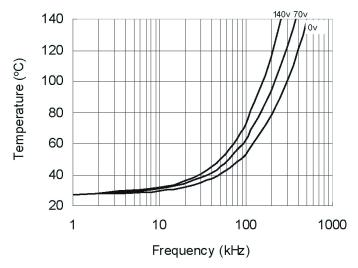
Figure 42. IRS21814s vs. Frequency (IRFPE50),  $\rm R_{\rm gate}$  =10  $\Omega, \, \rm V_{\rm cc}$  =15 V
