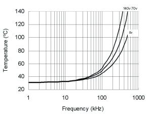
Figure 37. IRS2181s vs. Frequency (IRFBC40),  $R_{\text{nate}} \!=\! \! 15~\Omega,\, V_{\text{CC}} \! =\! \! 15~V$
