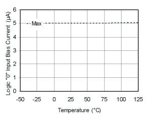
Figure 22A. Logic "0" Input Bias Curremt vs. Temperature
