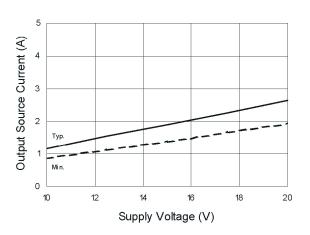
Figure 25B. Output Source Current vs. Supply Voltage
