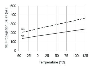
Figure 8A. SD Propagation Delay vs. Temperature
