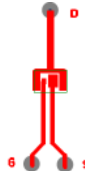
⑩ Mounted on minimum footprint full size board with metalized back and with small clip heatsink (still air)
