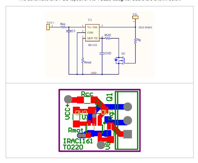
The daughter card shown above is designed to allow easy retrofit in existing systems with minimal system changes. The component values are recommended but user has freedom to change them per application requirement.
