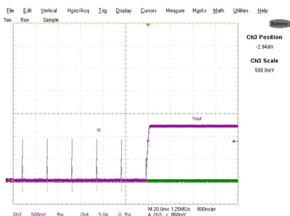
Figure 36 Short circuit (Hiccup) Recovery, SS_Select = Float, Ch3:V out , Ch4:I out
