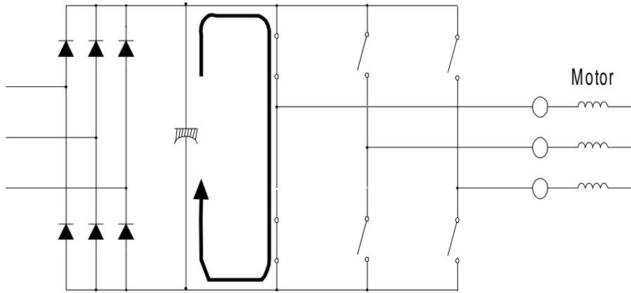
Figure 3: Current Flow during Shoot Through Mode
