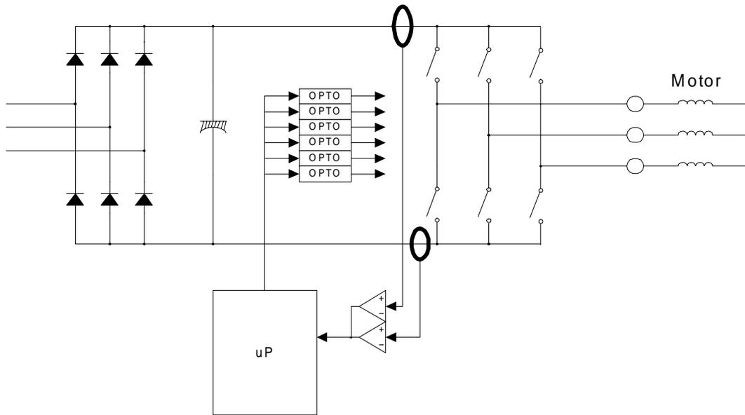
Figure 4: Overcurrent Protection in Floating Ground Reference System
