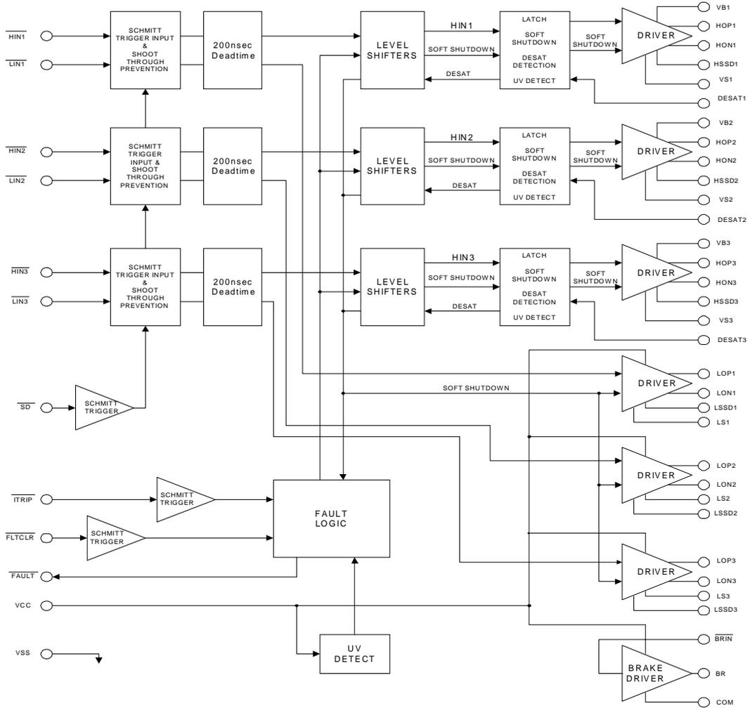
Figure 7: IR2137 Block Diagram
