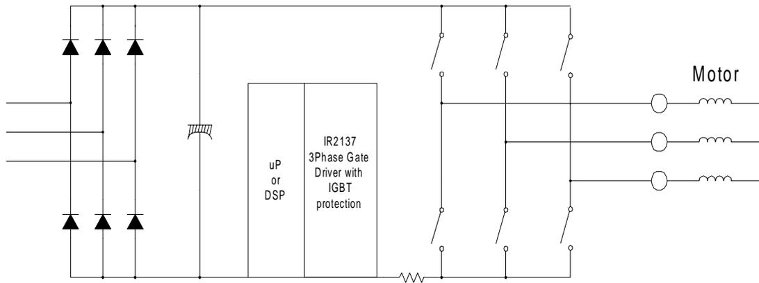
Figure 5: IR2137 Gate Driver with IGBT Overcurrent Protection
