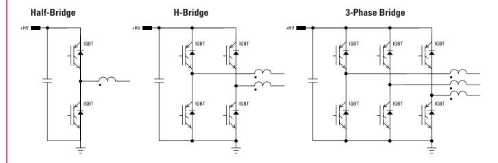
Traditionally, IGBT devices have excessive switching losses at higher frequencies used in UPS and solar inverters. IR's new Trench IGBT devices have low switching energy coupled with low conduction losses. These lower losses provide higher system efficiency, reducing the size of the magnetics and the cost of power generation to the end user.
