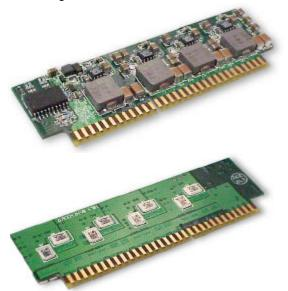
Fig. 4. Photograph of top and bottom side (heat sink over FETs on the bottom side not shown) of a VRM design (95mm X 31mm).
