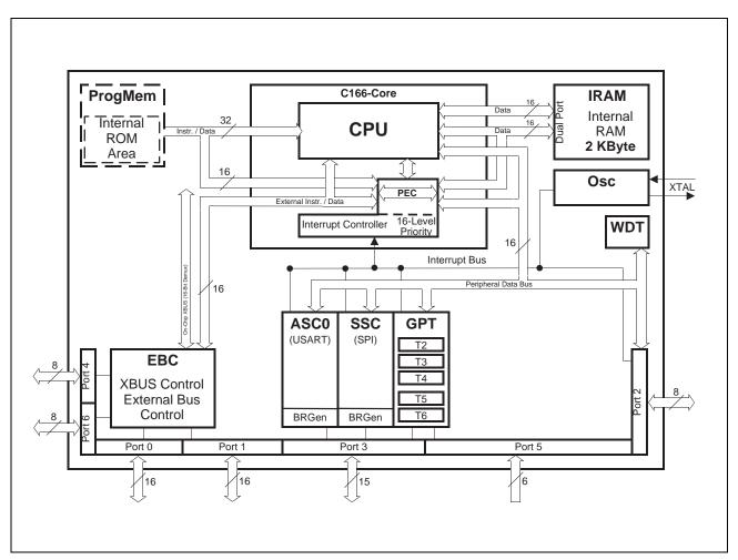
Figure 4 Block Diagram
