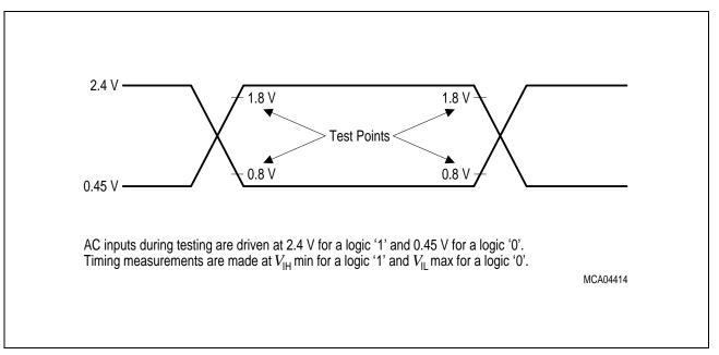
Figure 11 Input Output Waveforms
