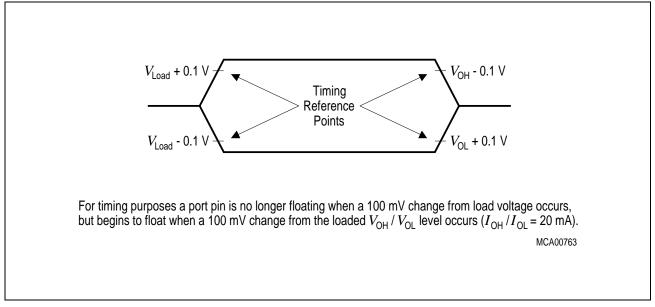
Figure 12 Float Waveforms
