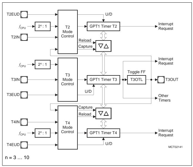
Figure 6 Block Diagram of GPT1
