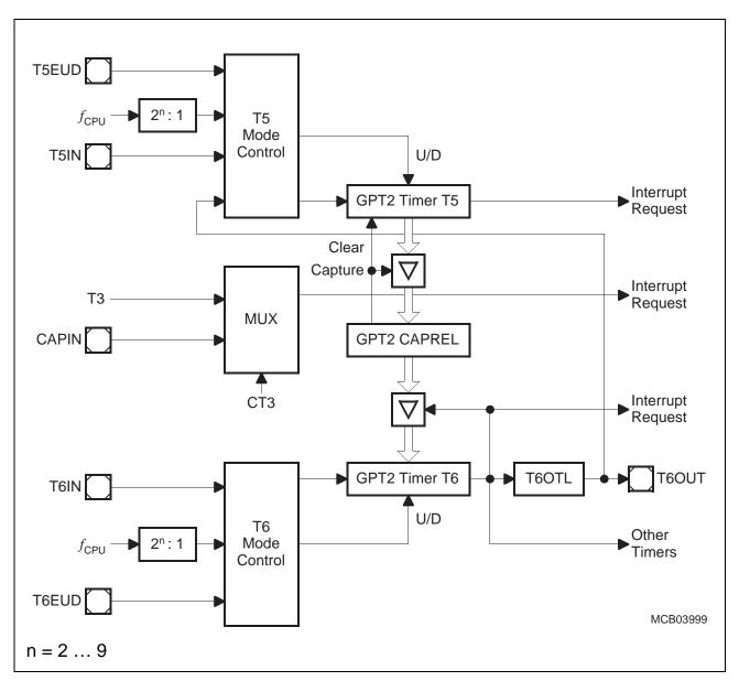
Figure 7 Block Diagram of GPT2
