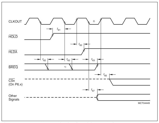
Figure 23 External Bus Arbitration, (Regaining the Bus)
