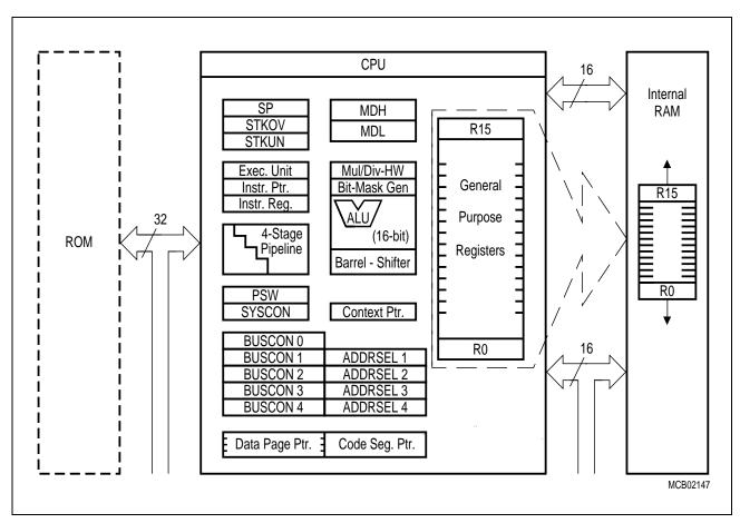
Figure 5 CPU Block Diagram
