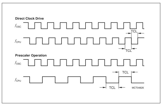
Figure 9 Generation Mechanisms for the CPU Clock
