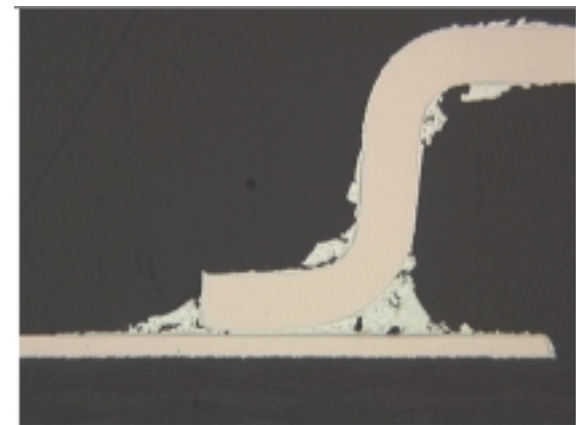
After 4000 T-cycles (SnAgCu on Ni/Au)
