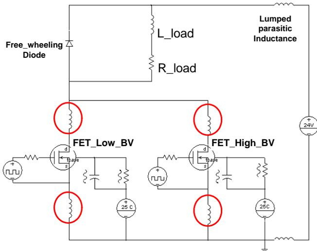
Figure 7: Circuit schematic for different terminal stray inductance
