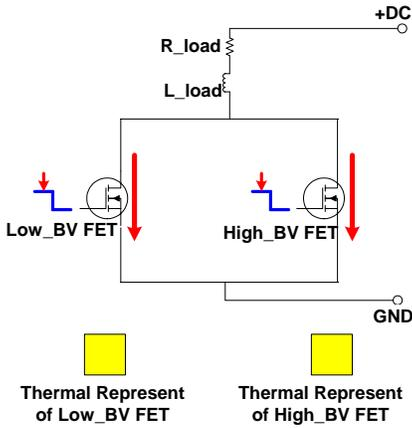
Figure 1-a: Current and thermal distribution during conduction
