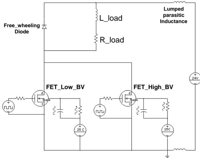
Figure 3: Circuit Schematic of two FETs in Parallel
