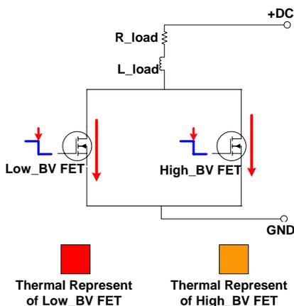
Figure 1-c: The rest of the turn-off process
