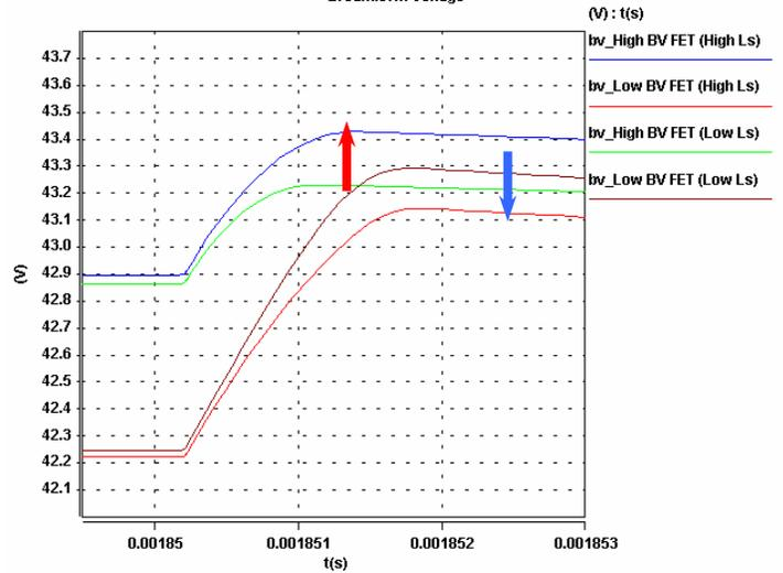
Figure 10: Breakdown Voltage (BV) Junction Temperature
