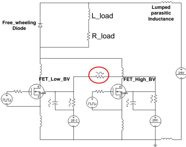
Figure 16: Circuit Schematic
