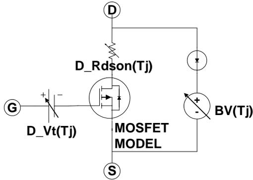
Figure 2: Avalanche model based on Quasi-dynamic model of IRF1404
