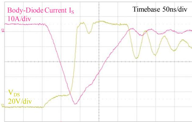
Fig. 6a Typical reverse-recovery waveform from device A1
