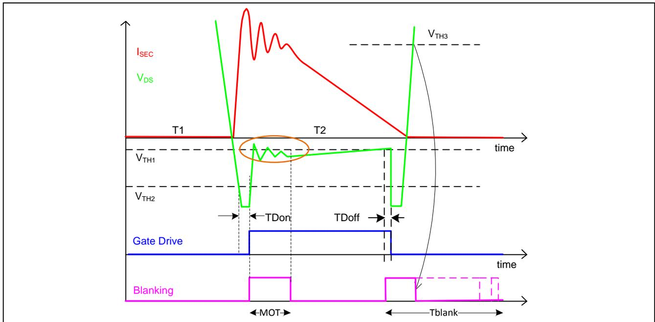
Figure 4 Secondary synchronous rectification waveforms of DCM/CrCM Flyback
