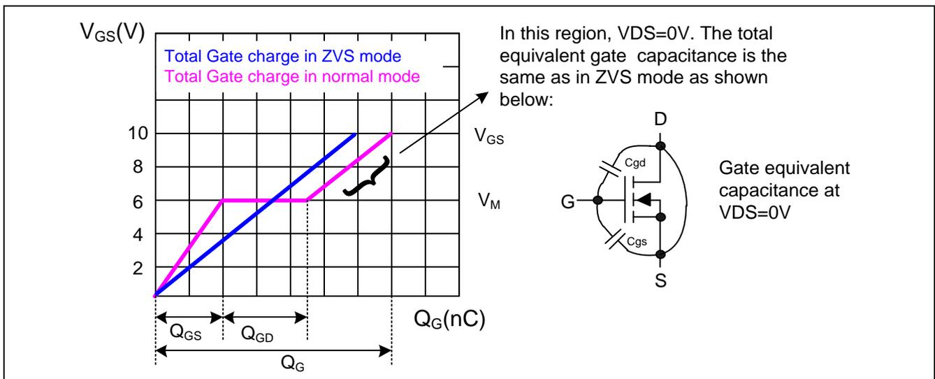
Figure 10 MOSFET gate equivalent capacitance in ZVS mode
