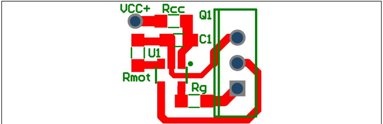
Figure 24 Single layer PCB example with TO-220 MOSFET
