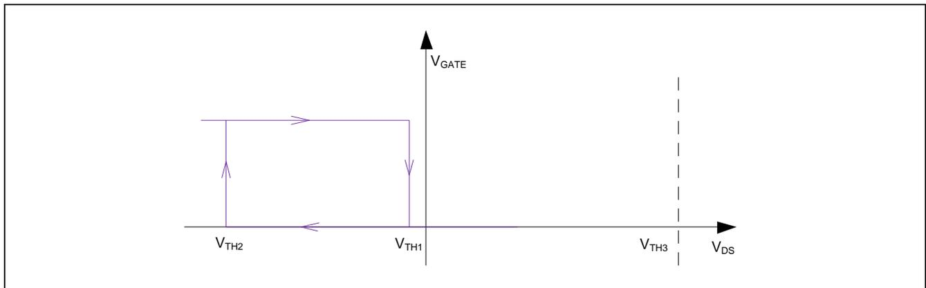
Figure 2 IR1161 SmartRectifier™ control IC voltage sensing thresholds
