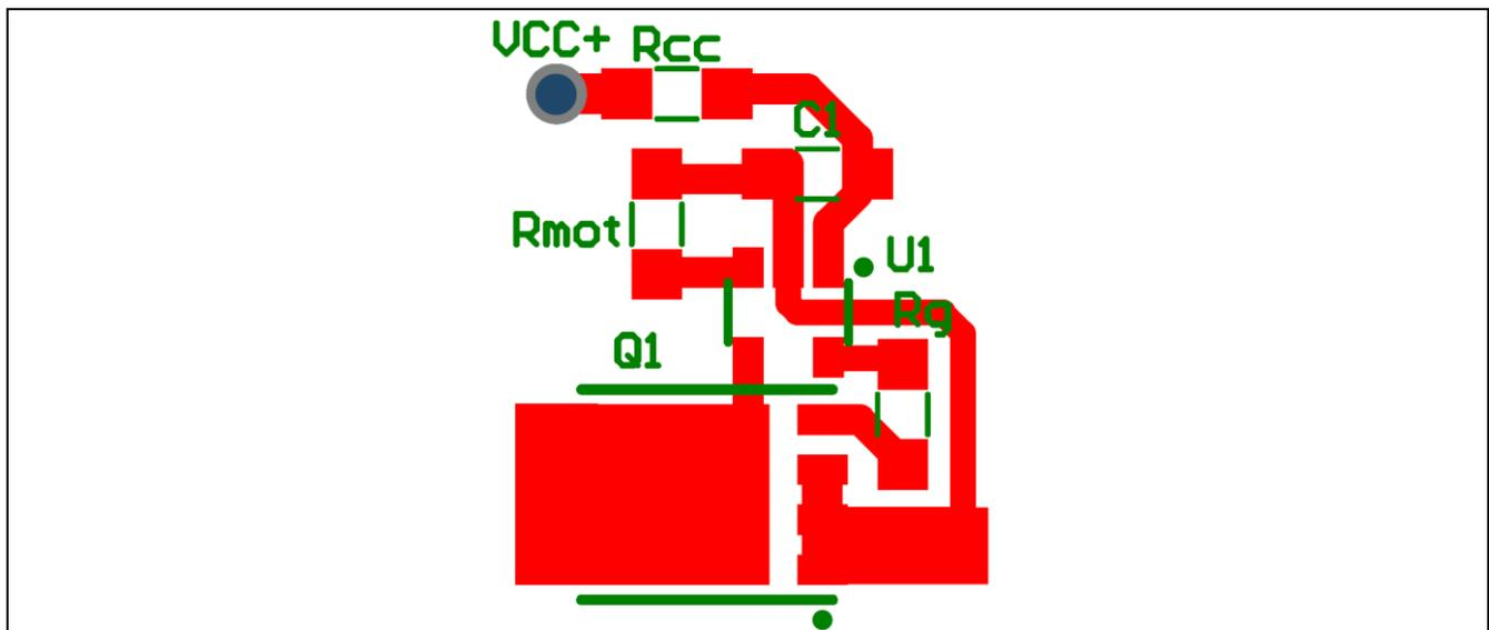
Figure 23 Single layer layout example with QFN MOSFET
