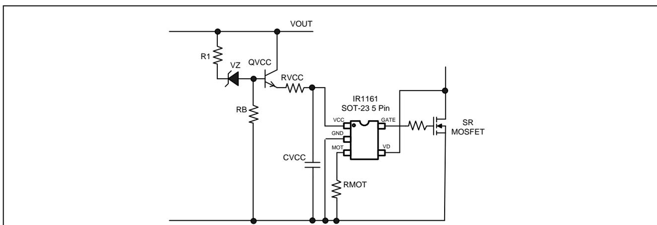
Figure 7 Simple VCC level shift supply circuit
