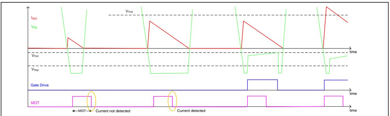
Figure 6 Gate drive resuming as load increases
