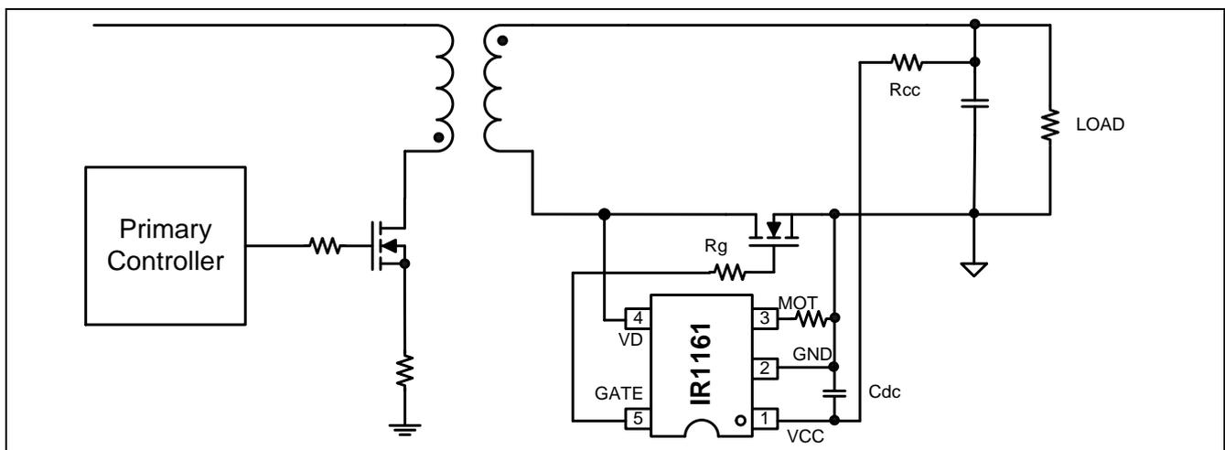
Figure 3 Flyback converter with synchronous output rectification
