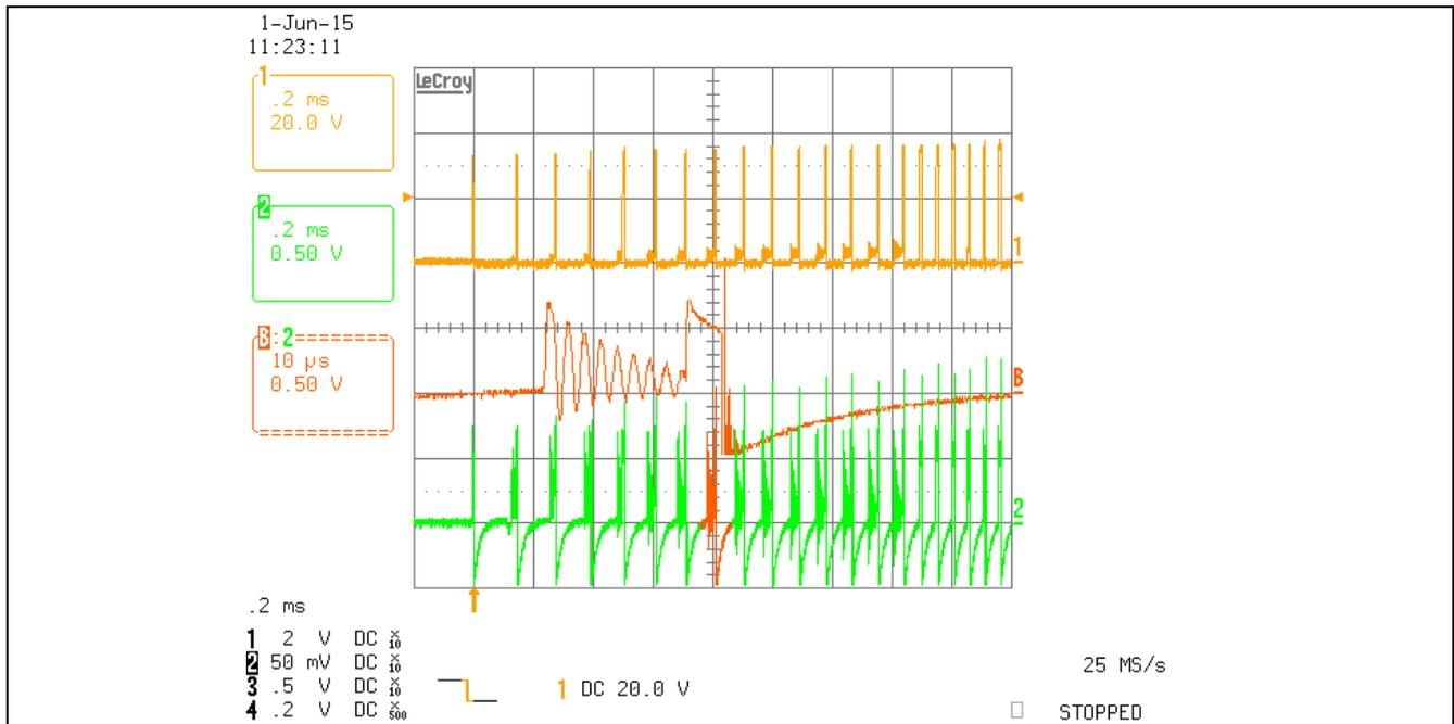
Figure 19 Gate waveform with clamping circuit during startup
