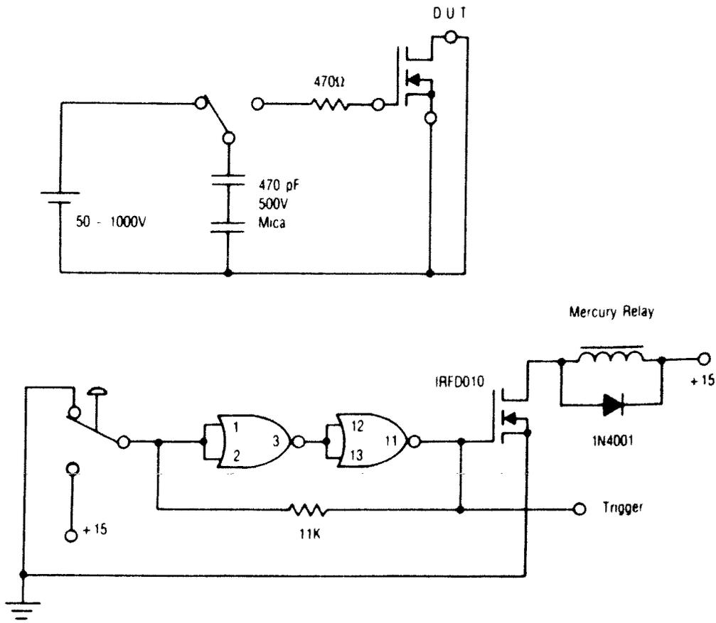
**Figure 6.** Schematic diagram of test circuit
