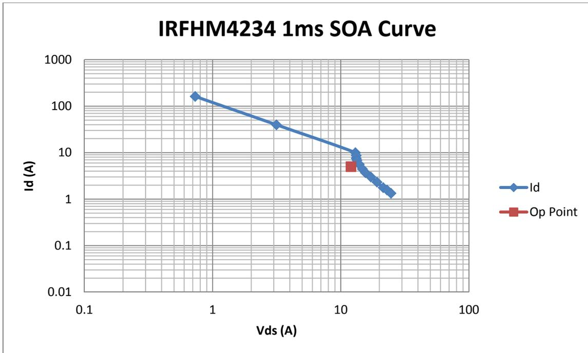
Figure 7 - IRFHM4234 1ms SOA compared to operating point
