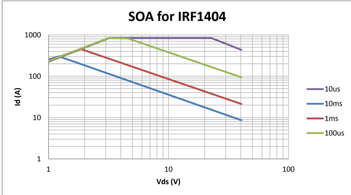
Figure 2 - SOA the IRF1404 (Planar MOSFET)
