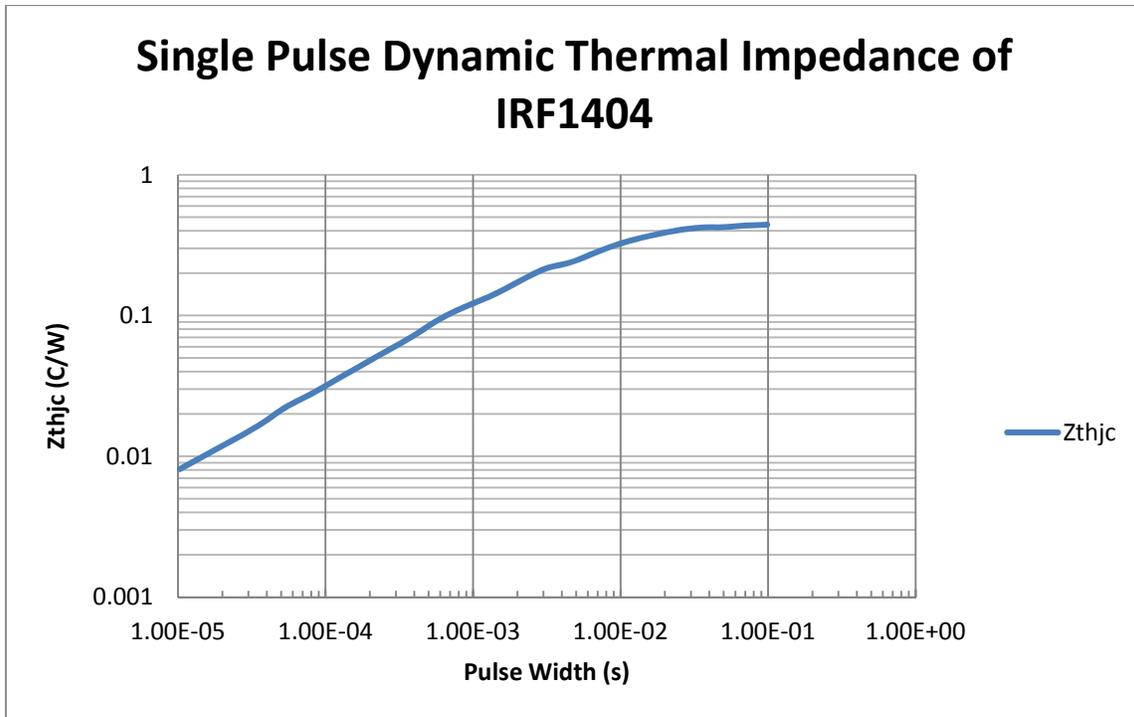
Figure 4 -  $Z_{thjc}$  of the IRF1404 Planar MOSFET
