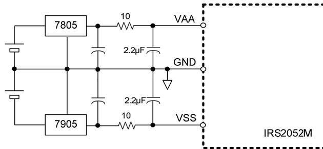
**Figure 28 Supplying  $V_{AA}$  and  $V_{SS}$  with External Regulators**
