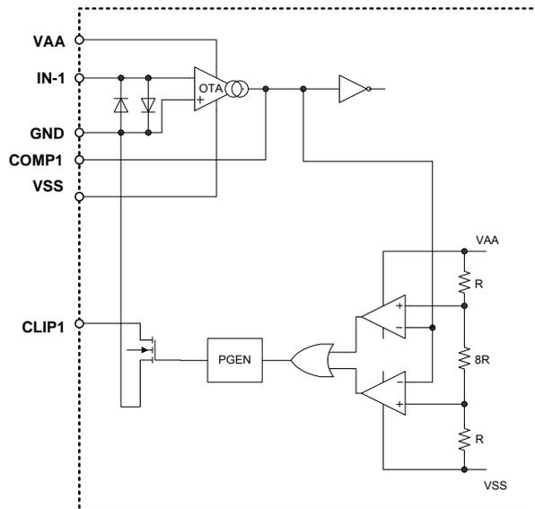
**Figure 24 Clipping Detection**
