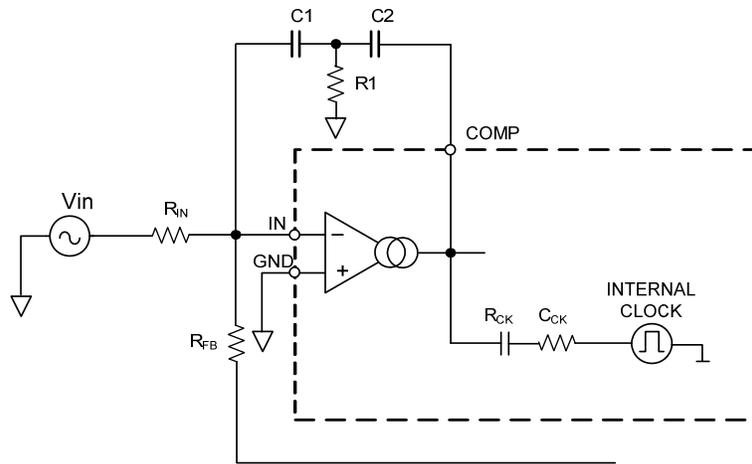
**Figure 4 Clock Synchronization**
