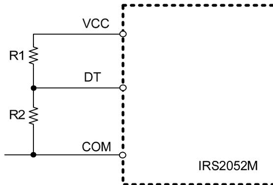
**Figure 27 External Voltage Divider for DT Pin**
