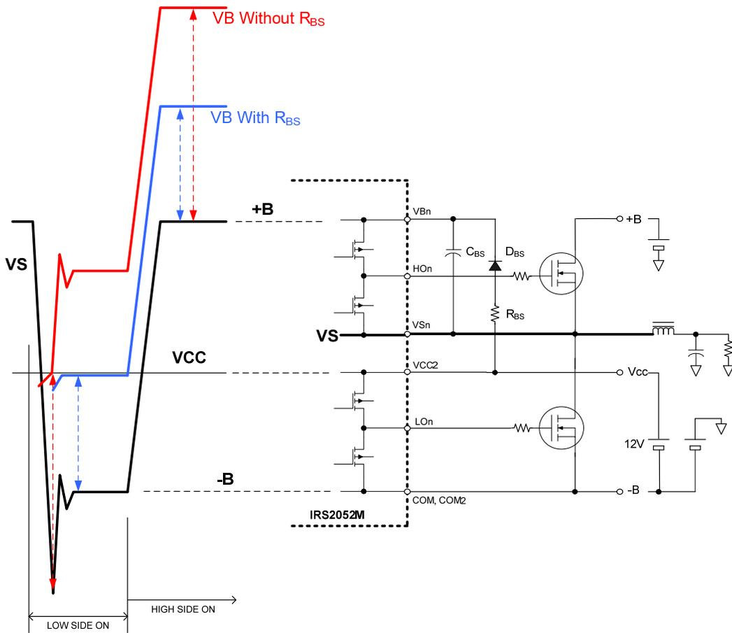
**Figure 35  $V_{BS}$  Charging With and Without  $R_{BS}$**
