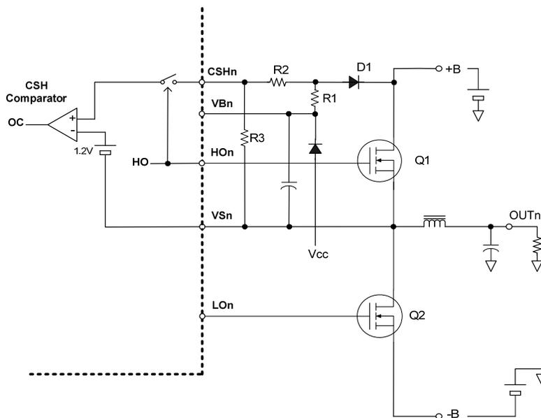
Figure 18 Programming High Side Over Current Threshold
