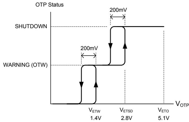
**Figure 21  $V_{OTP}$  vs. Over Temperature Protection Status**
