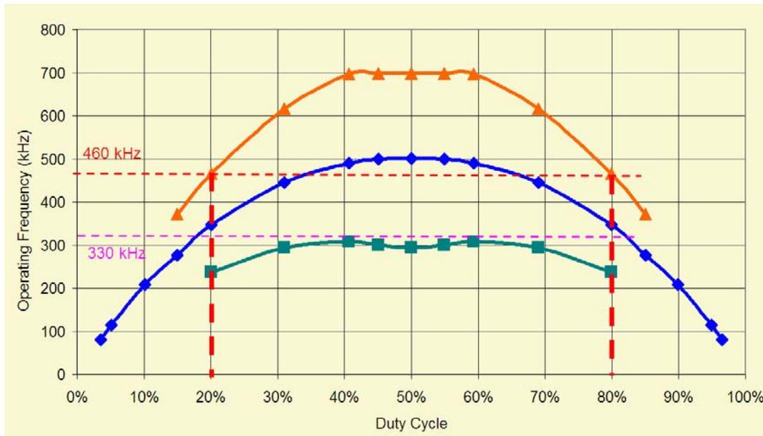
**Figure 6 Typical Lock Range to External Clock**
