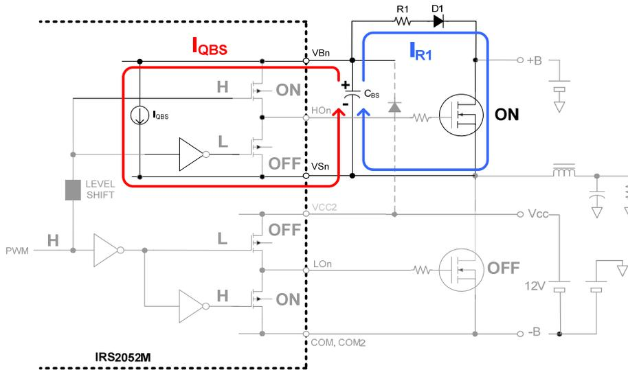
**Figure 34 C<sub>BS</sub> Discharging During High-side ON Period**
