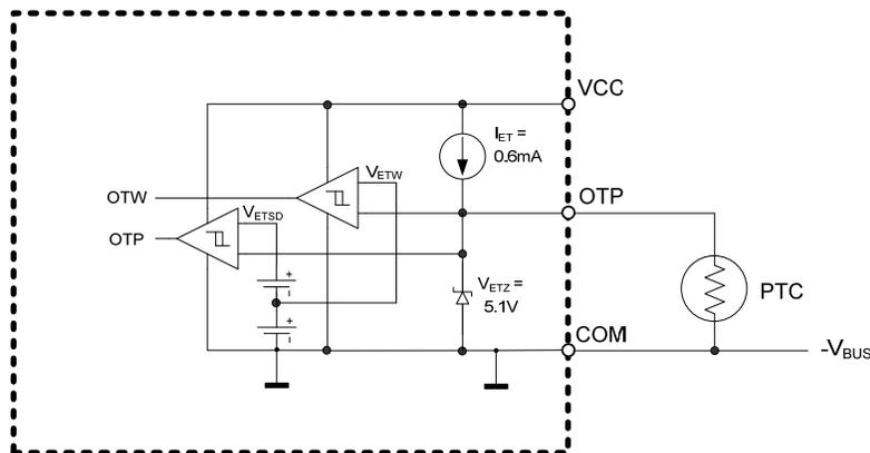
Figure 19 Over Temperature Protection (OTP) Input Structure
