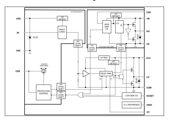
The IRS20955S and the IRS20957S share the same functional structure. In normal operating conditions, there are no functional changes between corresponding part numbers.
