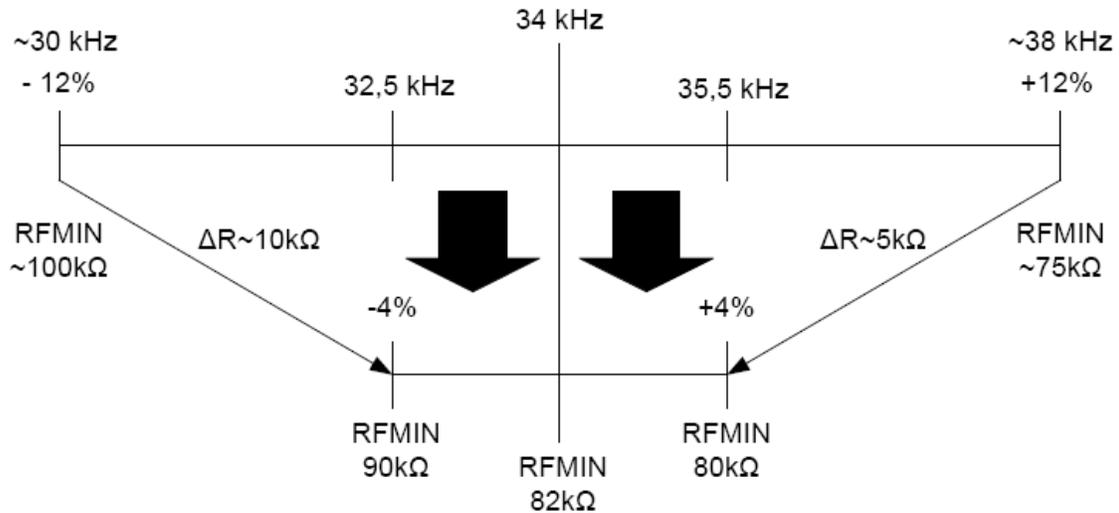
If the mean frequency of an IR2520D lot is between 30 and 32.5 kHz, decreasing RFMIN by 10 kΩ will bring the frequency back into the 34 kHz  $\pm 4\%$  range.
