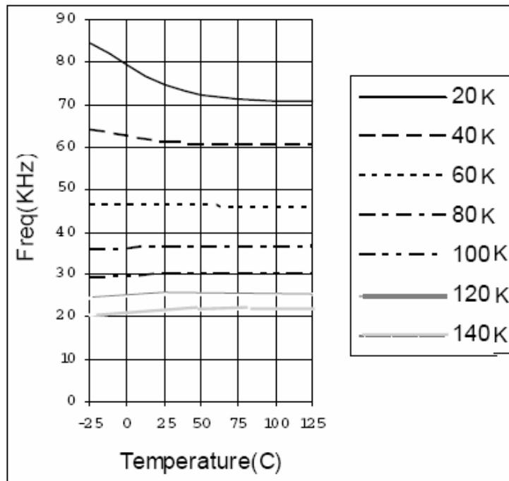
Fig. 14 Frequency vs R<sub>FMIN</sub> vs TEMP
