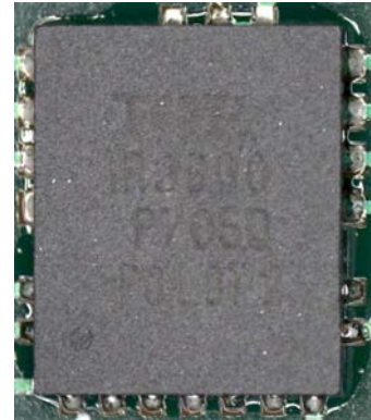
Figure 4 Self-centered with good solder fillets
