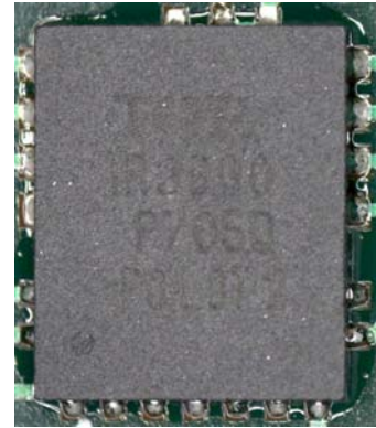
Figure 4 Self-centered with good solder fillets
