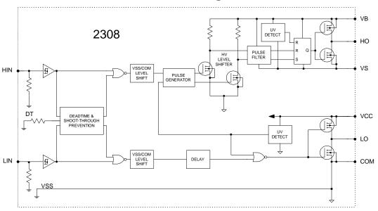
The IRS2308 and the IR2308 share the same block diagram. The functionality of the two ICs is the same.
