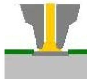
heres to the surface, due to the change in the effective length of the transducer, thus self limiting the bonding operation. If not correctly tuned the bonder may become super-sensitive to surface condition, on one hand, or continue to apply additional energy, which may then disrupt the bond or cause damage to the structures beneath the bonding pad.
