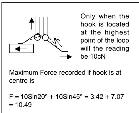
If the hook is placed in the centre of the wire, there is a much smaller angle at the die than at the substrate. Although there is no change in the wire or bonds the maximum reading will be 0.5cN greater. But, what is of greater concern is that, the forces are concentrated at the substrate, effectively reducing the force applied to the bond onto the die and making wire break on the substrate side more likely. Also both bonds may be weakened due to fatigue, at the heel of the bond.
