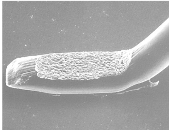
A tungsten “wedge” is fitted into an ultrasonic transducer. The wire is fed through a channel and under the front “foot”, as shown by the arrow in the figure opposite. The ultrasonic energy then simultaneously bonds and flattens the front end of the wire. The wedge then rises and moves back along the length of wire to just above the second bond position. Clamps positioned further back along the wire then close, so the wire is
