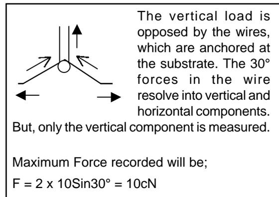
Note that as the loop height increases the reading will increase proportional to the Sin of the angle. So a flat wire of infinite length would give a reading close to zero and if both bonds were at the same location the reading could be as high as 20cN. The key element is that if the wire breaks, 10cN must have been applied between the hook and the bond on the side where the break took place.
