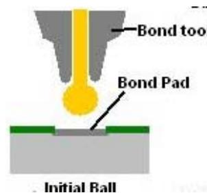
The ball, on the tip of the capillary, is then brought down onto the surface to be bonded, which has been preheated to the required temperature. Typically for thermo-sonic bonding this is between 100°C and 175°C.
