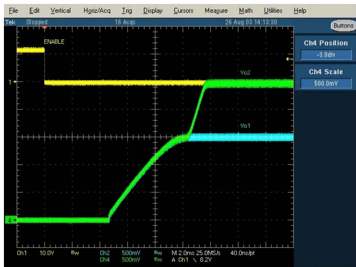
Figure 10 Simultaneous power-up using two soft start cap
