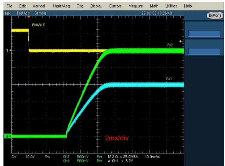
Figure 5 Ratiometric power-up using two soft start caps
