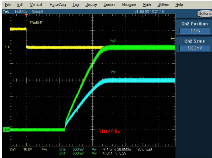
Figure 3 Ratiometric power-up using one soft start cap
