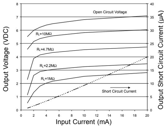
Figure 3. PVI5080N Typical Output Characteristics
