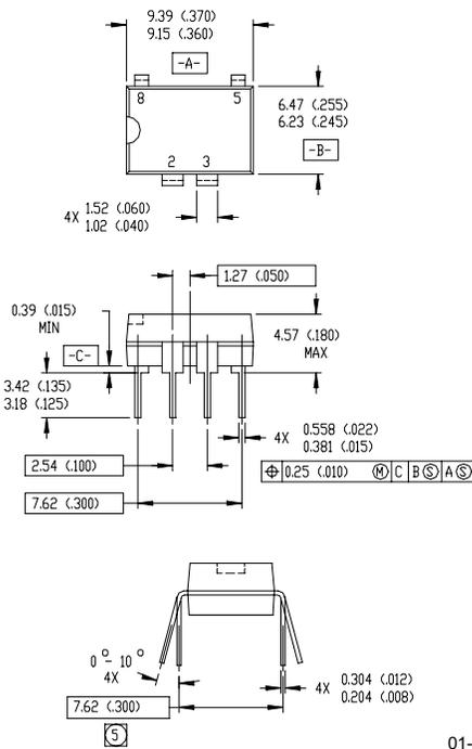
Fig. 1. Dual-in-Line Package
