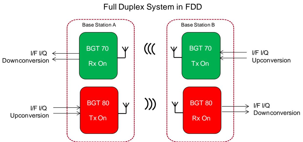
Figure 1: Typical application scenario in Mobile Backhauling using mmWave point-to-point link (can also be a TDD system)
