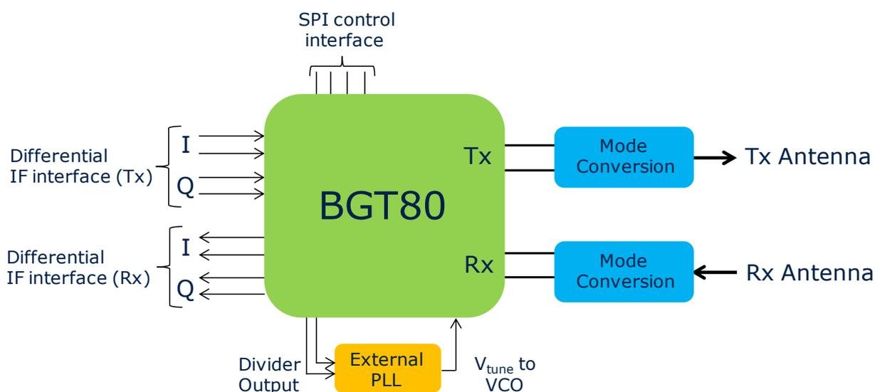
Figure 2: Block Diagram of Infineon's BGT80 (81-86GHz) Transceiver chipset
