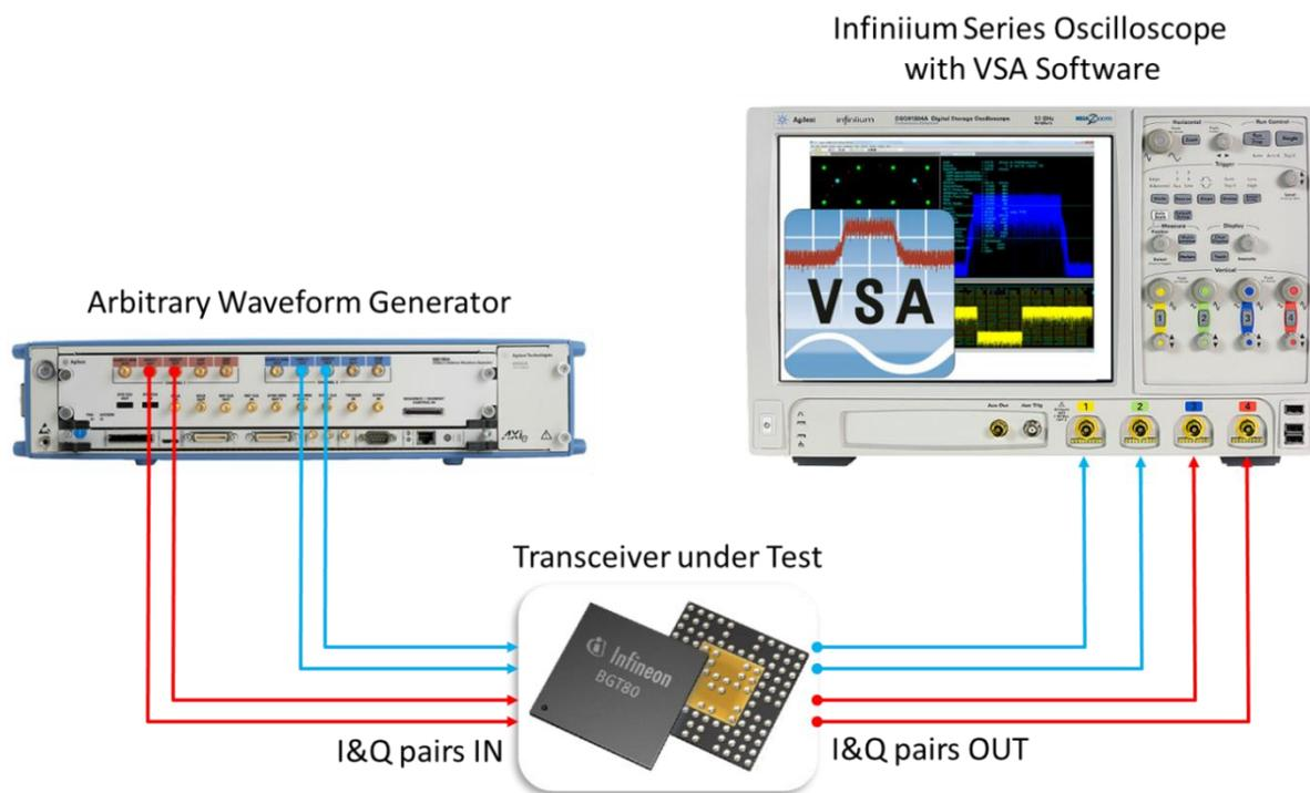
Figure 4: Basic Test and Measurement Setup for Transceiver Test
