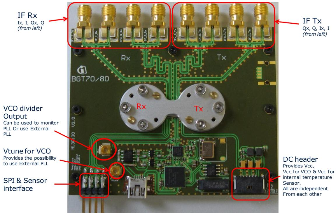
Figure 3: BGT80 Evaluation board used in link testing
