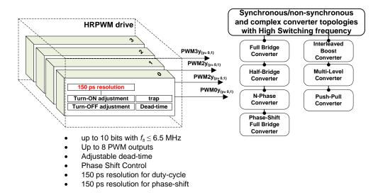
Figure 6 – HRPWM resources for generating the PWM
