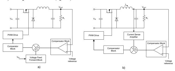
Figure 7 – Control loops: a) voltage control; b) current control
