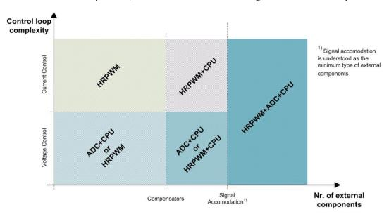
Figure 13 – Control Loop vs. External Components
