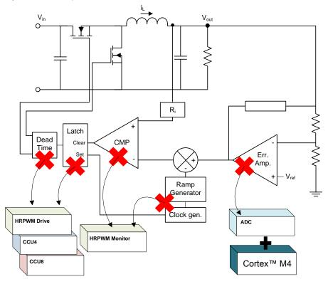
Figure 11 - Peak Current control with XMC4000
