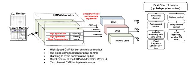
Figure 9 – HRPWM monitor resources for control loop implementation
