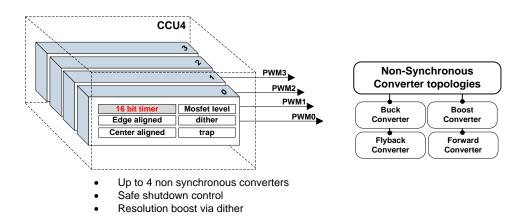
Figure 4 – CCU4 (Capture & Compare Unit 4) resources for generating the PWM
