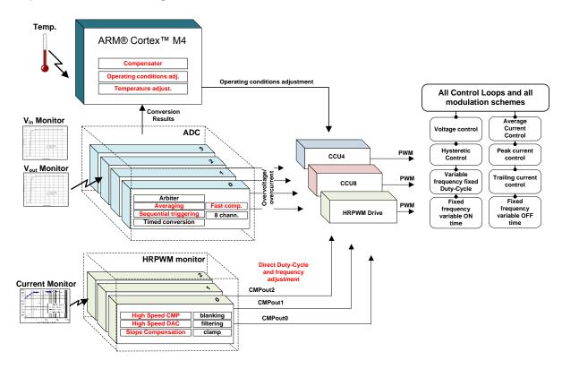
Figure 10 – XMC4000 resource organization for any type of control loop/power topology
