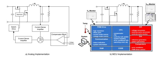
Figure 1 – Example of a Power Conversion application control with a microcontroller: a) Typical Analog Implementation; b) MCU implementation
