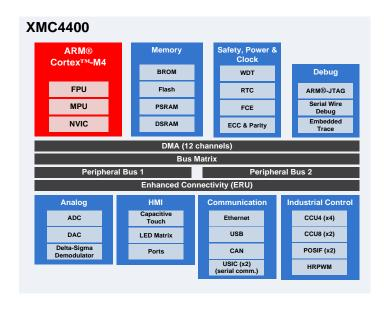
Figure 2 - XMC4400 Device Diagram
