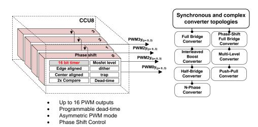
Figure 5 – CCU8 (Capture & Compare Unit 8) resources for generating the PWM
