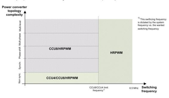
Figure 12 - Power Converter vs. Resources
