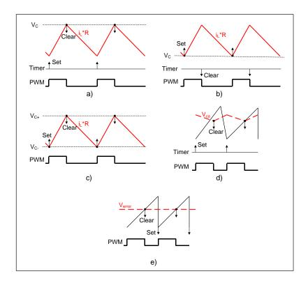
Figure 3 – Different modulation schemes: a) peak current control; b) valley current control; c) hysteretic control mode; d) average current control mode; e) voltage control mode
