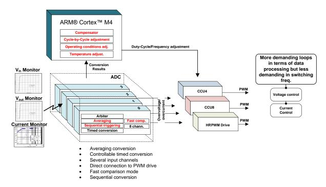
Figure 8 – ADC and ARM® Cortex™ M4 resources for control loop implementation
