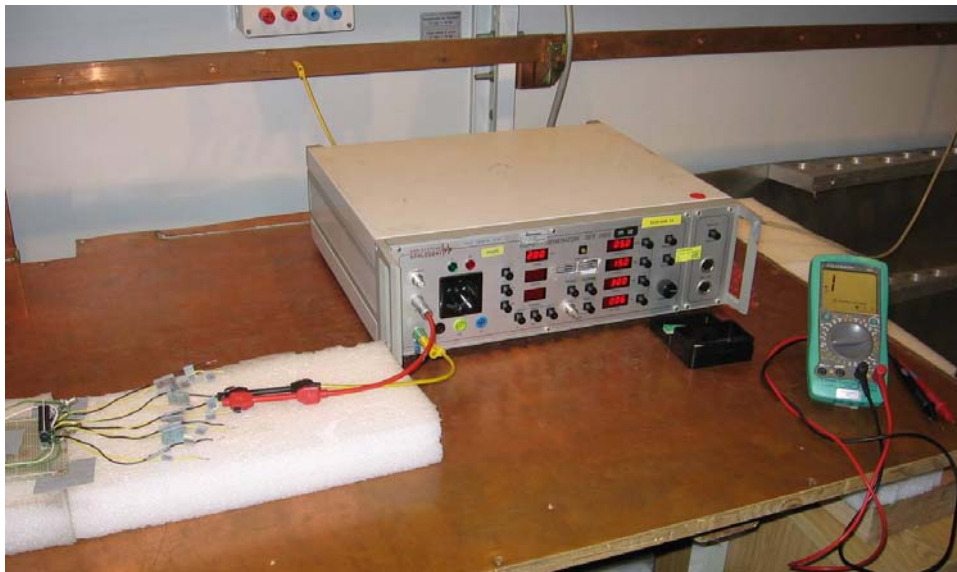
Figure 6-1: Test-Setup for the Burst tests
