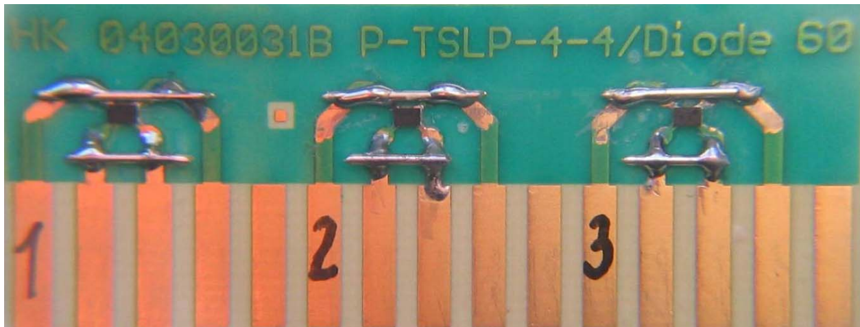
Figure 4-1: PCB with 3 pieces of RF ESD Protection Diode ESD0P4RFL
